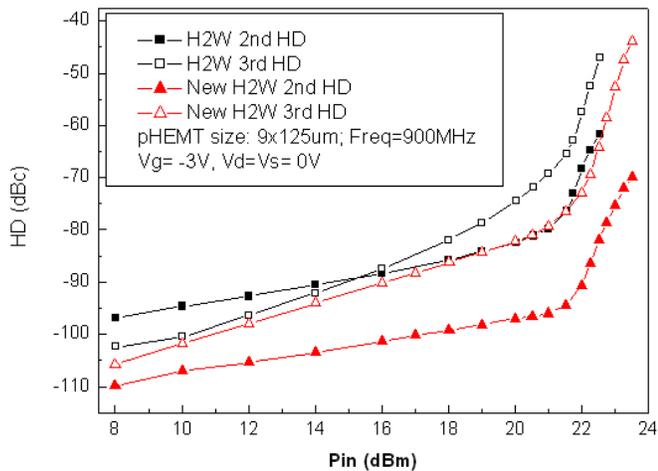
Fig4(b). H2W pHEMT switch harmonic comparison (off-state)
