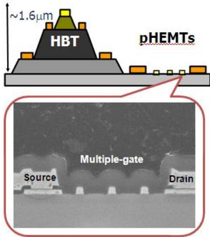
Fig1. New H2W construction and multiple gate cross-section image.
