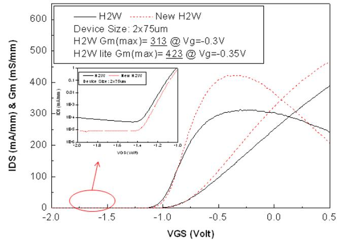
Fig2(a). pHEMT DC characteristic comparison of new H2W (Ids vs Vgs)
