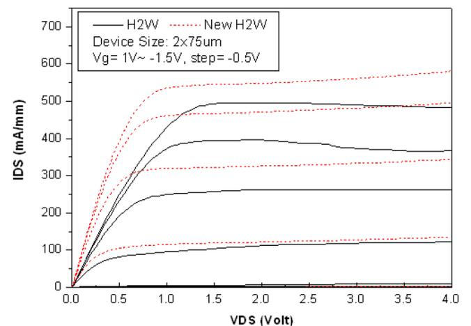
Fig2(b). pHEMT DC characteristic comparison of new H2W (Ids vs Vds)
