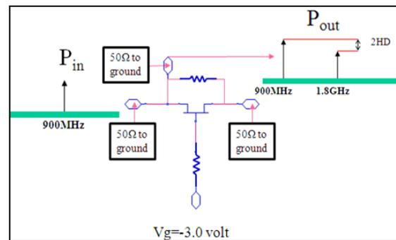
Fig4(a). Switch harmonic measurement method at off-state
