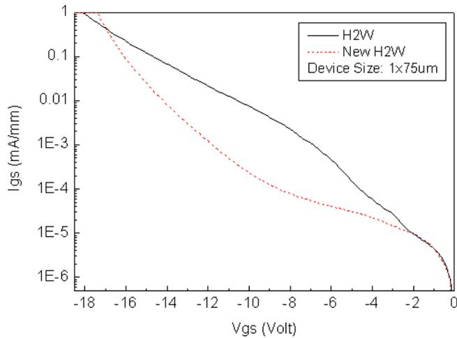
Fig3. New H2W Schottky gate characteristic comparison
