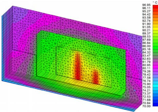
Fig. 6: Thermal model of power amplifier die in a 7×7 QFN package (epoxy/die junction layer shown).
