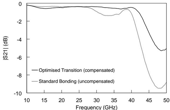
Fig. 3: Insertion loss of 4×4 mm QFN THRU.
