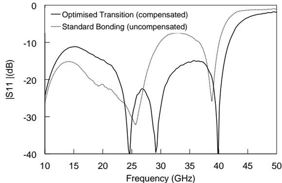
Fig. 4: Return loss of 4×4 mm QFN THRU.
