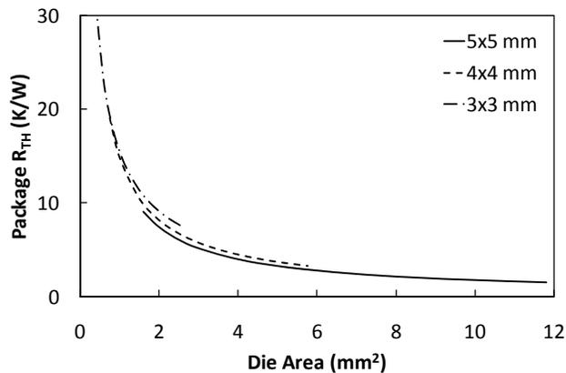
Fig. 5: QFN package thermal resistance vs. die area.
