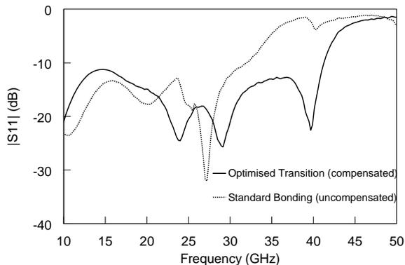
Fig. 2: Return loss of 3×3 mm QFN THRU.
