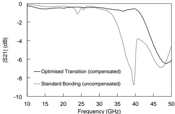
Fig. 1: Insertion loss of 3×3 mm QFN THRU.
