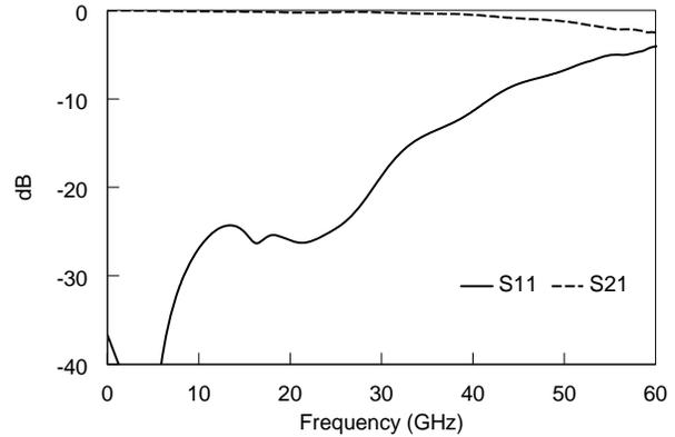
Fig. 7: Simulated transition for a 2.4 mm die in a 4×4 QFN package.
