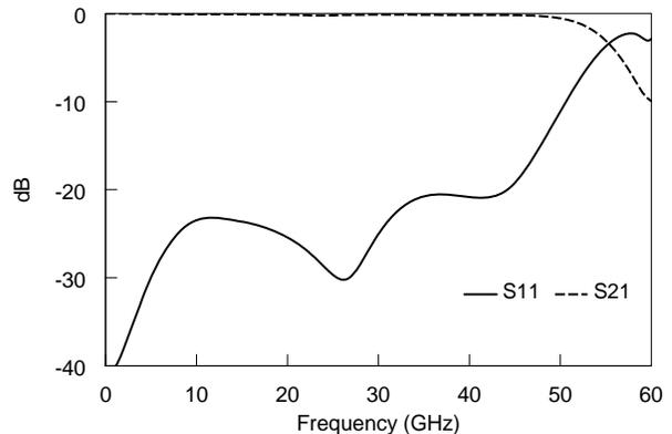
Fig. 8: Simulated transition for a 2.4 mm die in a custom 5×5 cavity laminate package.
