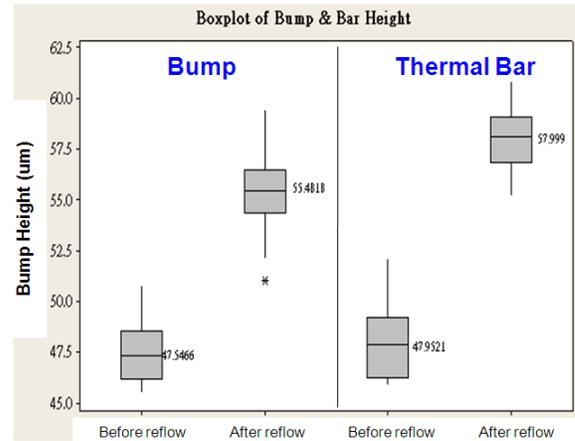
Figure 5. Bump height measured before and after solder reflow process for a chip design with a short thermal bar.
