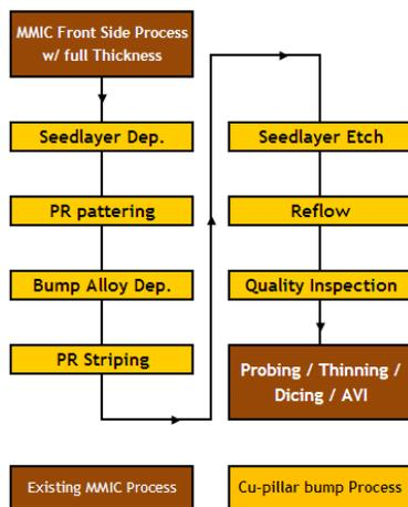
Figure 2. Typical Cu-pillar bump process flow
