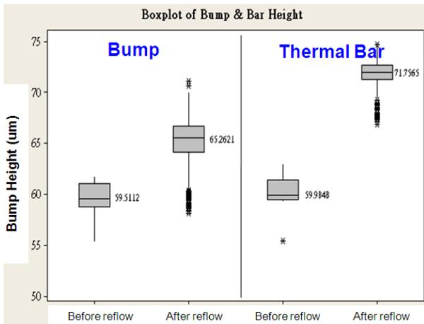
Figure 7. Bump height measured before and after solder reflow process for a chip design with a long thermal bar.
