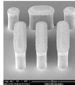
Figure 3. A Cu-pillar bump layout with thermal bars in the chip. Thermal bar can improve heat dissipation to ensure the chip's performance.
