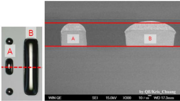
Figure 4. Cross-section shows different bump heights can be expected from different bump sizes although they are in the same chip.
