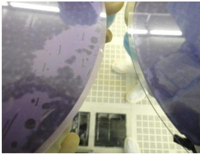
Figure 1. Chemical attack on adhesion materials after PR stripping process.
