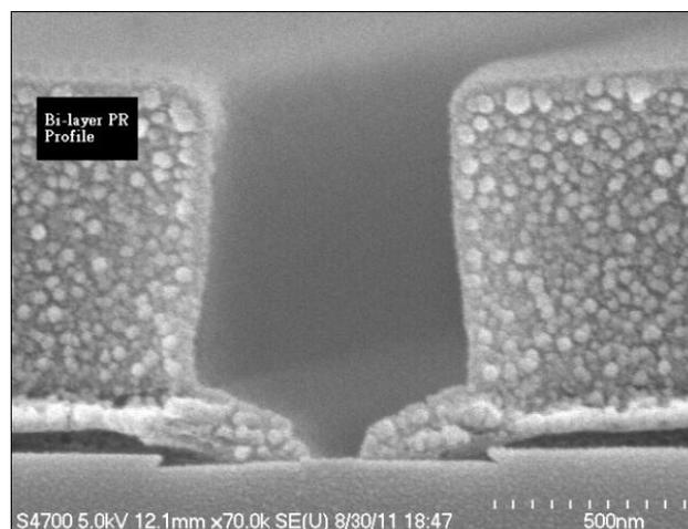
Figure 1, The bi-layer resistance profile of e-beam lithography technology.
