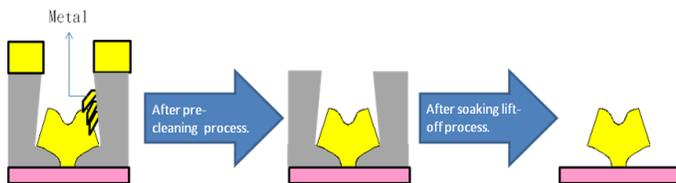
Figure 4, The concept of IPA spray type clean plus ACE soaking type clean
