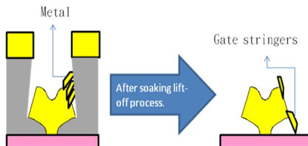
Figure 2, The mechanism of metal stringer.
