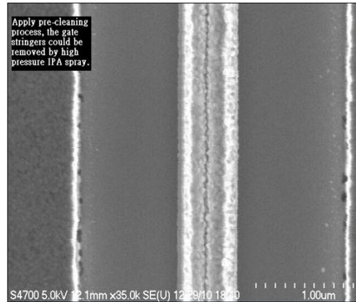
Figure 5, The SEM picture of the gate by using new lift-off process
