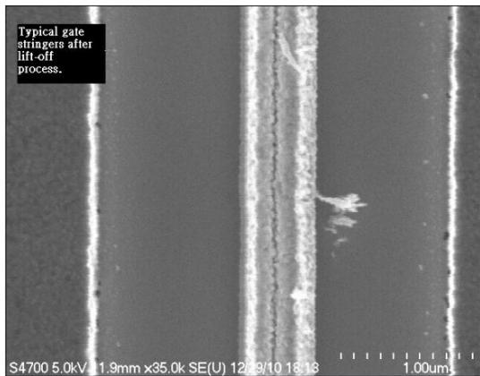
Figure 3, The photo of stringers on top of gate, and between gate and semiconductor
