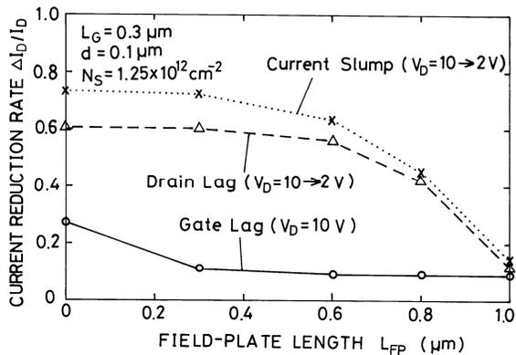
Fig.4 Current reduction rate  $\Delta I_D/I_D$  due to current slump, drain lag or gate lag for GaAs MESFETs, with field plate length  $L_{FP}$  as a parameter.  $d = 0.1 \mu\text{m}$ .  $N_S = 1.25 \times 10^{12} \text{cm}^{-2}$ .
