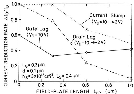
Fig.6 Current reduction rate  $\Delta I_D/I_D$  due to current slump, drain lag or gate lag for GaAs MESFETs, with field plate length  $L_{FP}$  as a parameter.  $d = 0.1 \mu\text{m}$ .  $N_S = 3 \times 10^{12} \text{cm}^{-2}$  and the surface-state length is  $0.4 \mu\text{m}$ .
