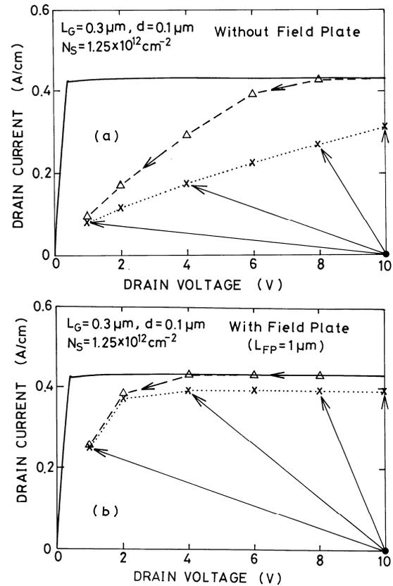
Fig.3 Steady-state  $I$ - $V$  curves ( $V_G = 0$  V; solid lines) and quasi-pulsed  $I$ - $V$  curves ( $\Delta$ ,  $x$ ) of GaAs MESFETs with surface states.  $N_S = 1.25 \times 10^{12} \text{ cm}^{-2}$ . (a) Without field plate, (b) with  $1 \mu\text{m}$ -length field plate.  $d = 0.1 \mu\text{m}$ . ( $\Delta$ ): Only  $V_D$  is changed from 10 V ( $t = 10^{-8}$  sec), ( $x$ ):  $V_D$  is lowered from 10 V and  $V_G$  is changed from  $V_{th}$  to 0 V ( $t = 10^{-8}$  sec).
