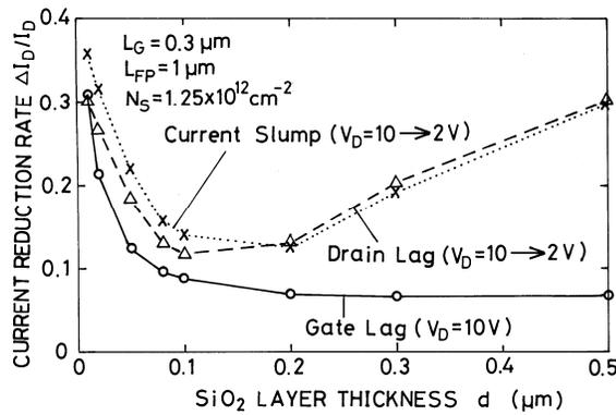
Fig.5 Current reduction rate  $\Delta I_D/I_D$  due to current slump, drain lag or gate lag for GaAs MESFETs, with  $\text{SiO}_2$  layer thickness  $d$  as a parameter.  $L_{FP} = 1 \mu\text{m}$ .  $N_S = 1.25 \times 10^{12} \text{cm}^{-2}$ .
