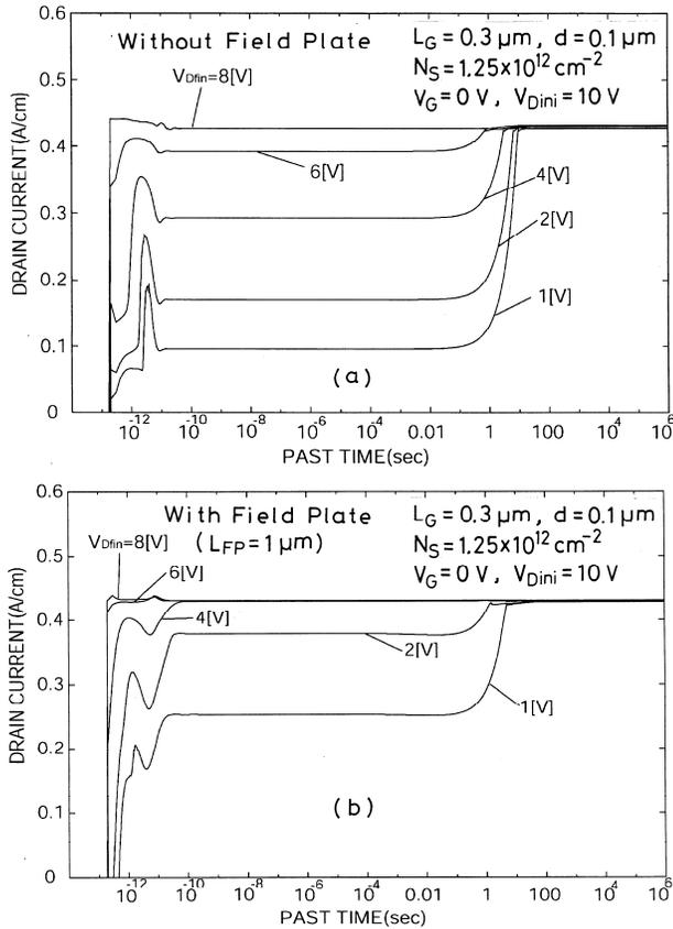
Fig.2 Calculated drain-current responses of GaAs MESFETs with surface states when  $V_D$  is lowered abruptly from 10 V to  $V_{Dfin}$ , while  $V_G$  is kept constant at 0 V.  $N_S = 1.25 \times 10^{12} \text{ cm}^{-2}$ . (a) Without field plate, (b) with field plate ( $L_{FP} = 1 \mu\text{m}$ ,  $d = 0.1 \mu\text{m}$ ).
