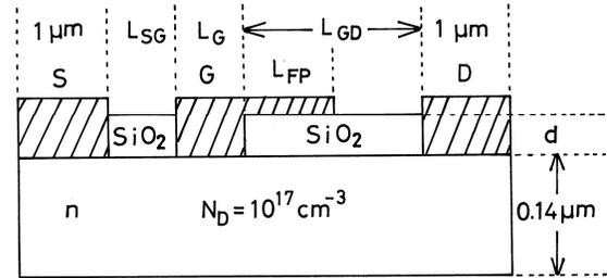
Fig.1 Device structure analyzed in this study.
