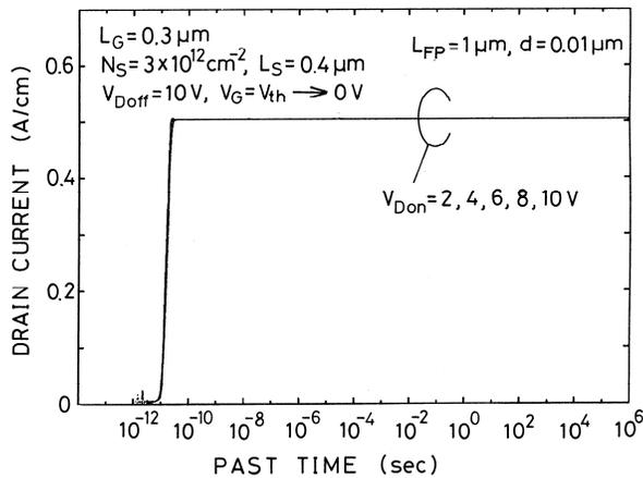
Fig.7 Calculated turn-on characteristics for  $L_{FP} = 1 \mu\text{m}$  and  $d = 0.01 \mu\text{m}$  when  $V_D$  is lowered abruptly from 10 V to  $V_{Don}$  and  $V_G$  is changed from  $V_{th}$  to 0 V.  $N_S = 3 \times 10^{12} \text{cm}^{-2}$  and the surface-state length is 0.4  $\mu\text{m}$ .
