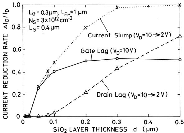
Fig.8 Current reduction rate  $\Delta I_D/I_D$  due to current slump, drain lag or gate lag for GaAs MESFETs, with  $\text{SiO}_2$  layer thickness  $d$  as a parameter.  $L_{FP} = 1 \mu\text{m}$ .  $N_S = 3 \times 10^{12} \text{cm}^{-2}$  and the surface-state length is 0.4  $\mu\text{m}$ .
