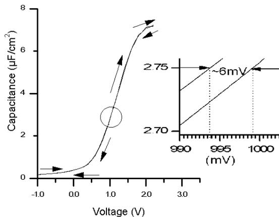
Figure 4: A CV sweep of the thinner at 20 KHz revealed the MOSCAP displayed little hysteresis.
