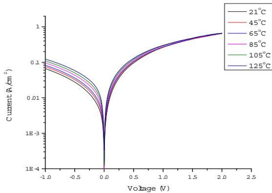
Figure 8: Variations in temperature had little effect on the thinner gate oxide consistent with direct tunneling.
