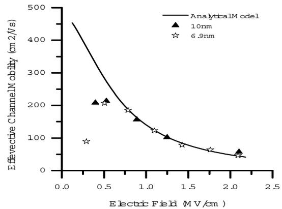
Figure 6: The effective electron mobility through the GaN is consistent for both the 6.9nm and 10 nm oxides.
