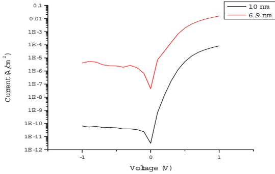
Figure 7: The gate oxides display near ideal tunneling current that scales appropriately with oxide thickness.
