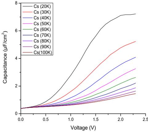
Figure 2: Spreading effects lower the effective capacitance as the measurement frequency increased. Lower frequencies produce the best reflection of the actual capacitance of the dielectric film.
