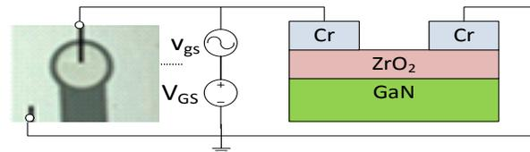
Figure 1: The top view of a typical  $100 \times 1000 \mu\text{m}$  MOSCAP taken with a confocal microscope, an illustrated cross section with test set up for typical measurements..
