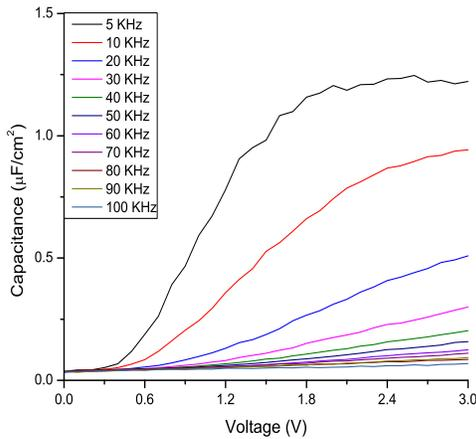
Figure 3: The capacitance density was  $1.2\mu\text{F/cm}^2$  at 5 KHz. Spreading effects were also observed on the thicker sample.
