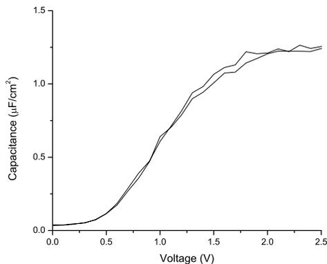
Figure 5: A CV sweep of the thicker MOSCAP at 5 KHz revealed a larger hysteresis than the thinner sample displayed.
