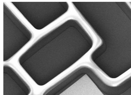
Figure 4: Wall Distortion After Cure
