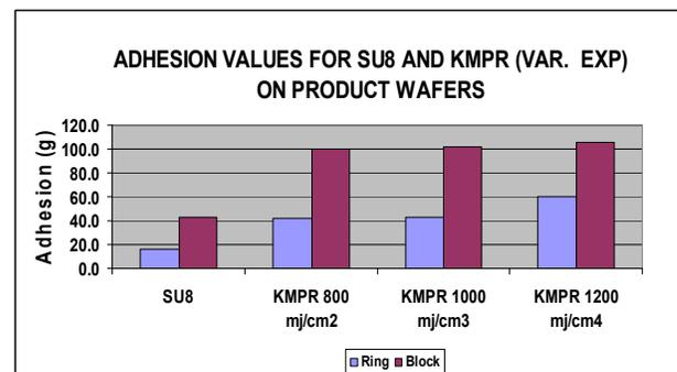
Figure 3: Adhesion Data for KMPR vs. SU8 on Product Wafers
