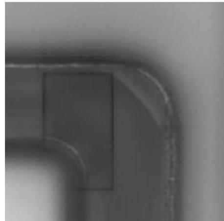
Figure 1: Delamination
