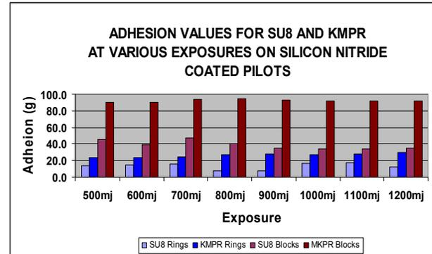
Figure 2: Adhesion Data for KMPR vs. SU8 on Pilot Wafers
