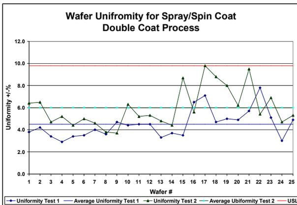
For the two tests, the overall average resist thickness was  $71.4 \mu$  and the overall average uniformity was  $\pm 5.3 \%$ . The average uniformity for Test 1 was  $\pm 4.5 \%$  and Test 2 was  $\pm 6.0 \%$ .
