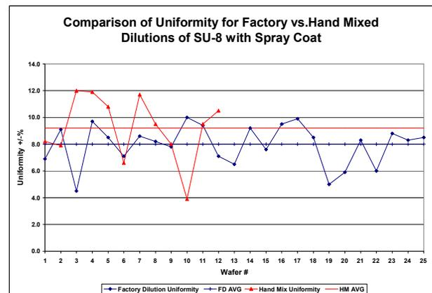
The current process for double spin coating is specified at  $77.4 \pm 4.8\mu$  for the average wafer thickness and uniformity less than or equal to  $\pm 9.8\%$ . The average thickness is averaging  $76.7\mu$  and the uniformity is averaging  $\pm 5.4\%$  with the current process. The following charts show the average resist thickness per wafer and the uniformity per wafer for two tests processed using the spin coat/spray coat double coat process.
