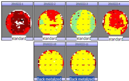
**Figure 5 Back-metallized wafers (10, 11) have much more uniform wafer maps than standard wafers (1 through 4).**
