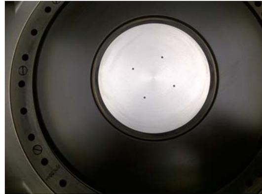
**Figure 4 Wafer chuck of the etch tool with the four lift-pins.**
