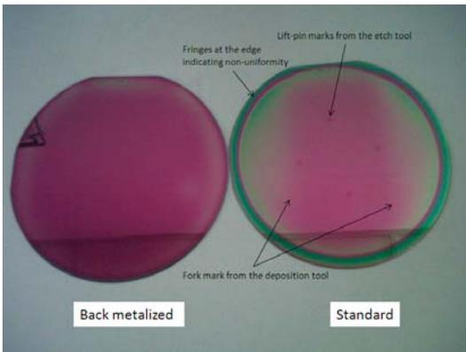
**Figure 2 Comparison of back-metalized wafer and standard wafer after nitride etch**
