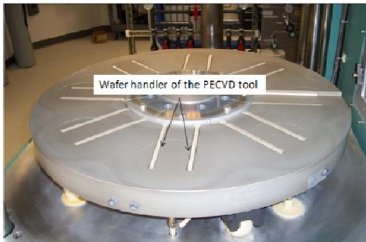
**Figure 3 Wafer handler of the Novellus PECVD tool.**
