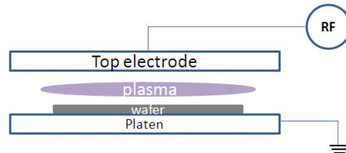
Figure 1 A typical parallel plate RIE system.
