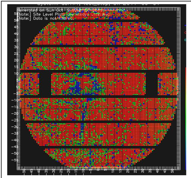
**Fig 1:** DC die sort wafer map showing die failing test. The failure pattern gave clues to the source of failures. Failing die were analyzed and a focused ion-beam (FIB) cross-section is shown in Fig 2.
