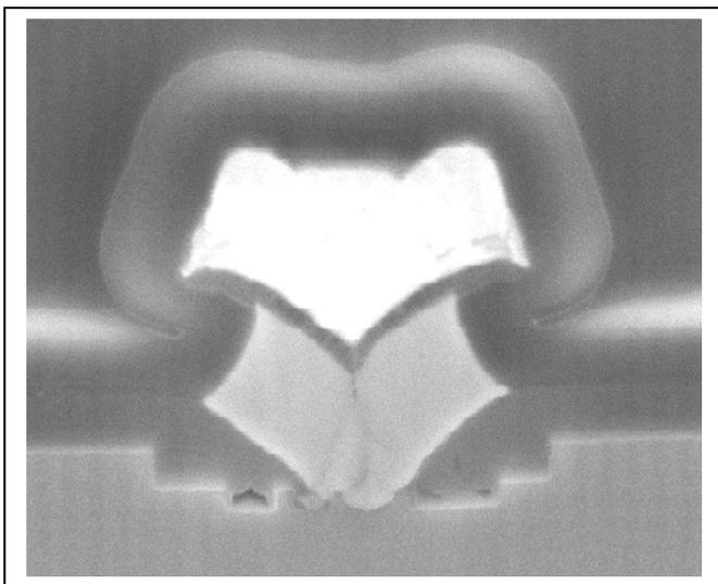
**Fig 2:** FIB cross-section showing root cause of the DC die sort test failures causing yield loss shown in the wafer map in Fig 1. Incomplete formation of the FET is observed causing excessive Drain off-current.
