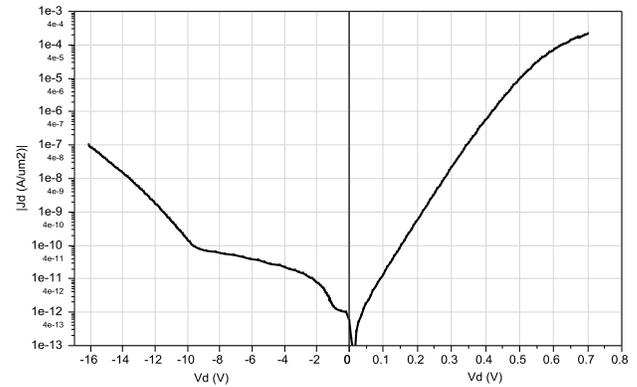
Figure 3. Forward and reverse I-V curves of the TaN Schottky diode (absolute values).
