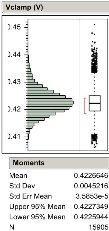
Figure 2. Distribution of measured diode turn-on voltage across a large sample.
