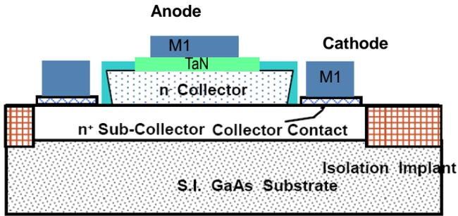
Figure 1. Schematic of the TaN Schottky diode.
