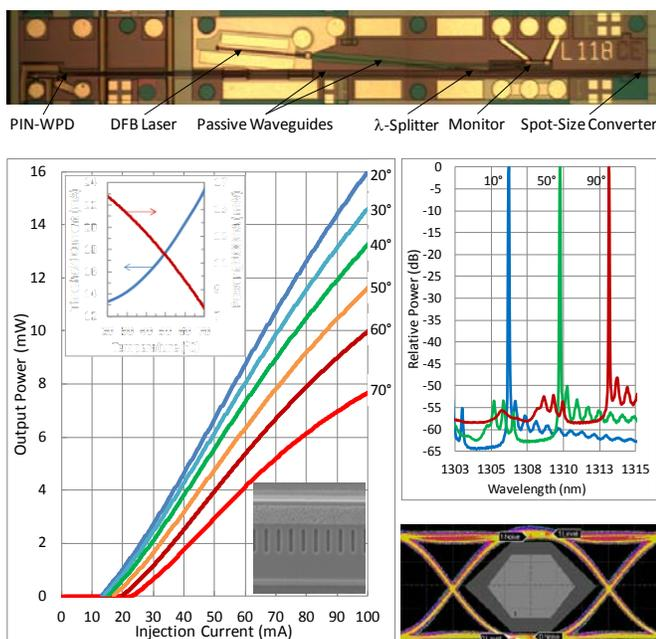
**Figure 1** Diplexer PIC for ONU transceiver applications in FTTH networks. Top – optical microscope image; bottom – key performance features of the on-chip DFB laser. Shown in the bottom right corner insert to the light-current characteristic plot on the left is the scanning electron microscope image of the vertically-coupled surface-etched grating, which makes the laser's DFB cavity.
