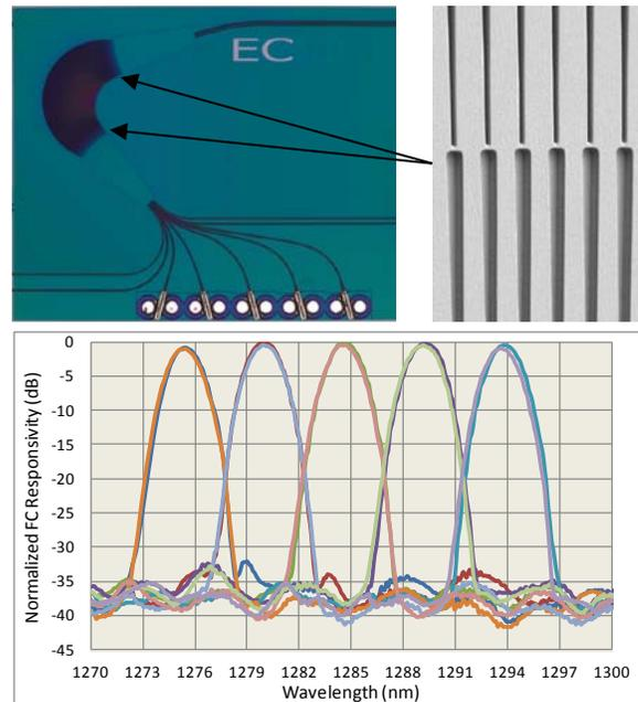
**Figure 2** 5x25G / 800GHz WDM receiver PIC for high-capacity transport OI. Top – optical microscope image of the die (left) and scanning electron microscope image of the shallow etch – deep etch waveguide junction; bottom – normalized fiber-coupled responsivity spectra in TE and TM polarizations.
