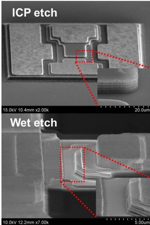
Figure 1. The scanning electron microscopic image of RCLET
