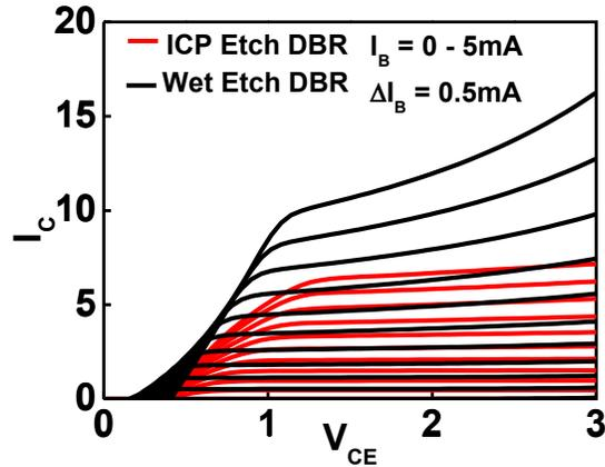
Figure 2. The Family Curve of RCLET with ICP and wet etching DBR.
