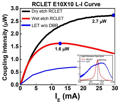
Fig. 3. The intensity versus emitter injection current of RCLET and LET
