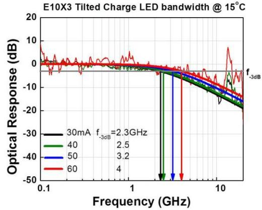
Figure 4. The frequency response of RCLET with 4 GHz bandwidth
