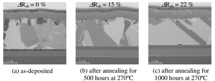
Figure 5. Cross section SIM images of sample C. The Pd film of sample C is the electroplating film with a crystalline adjuster.
