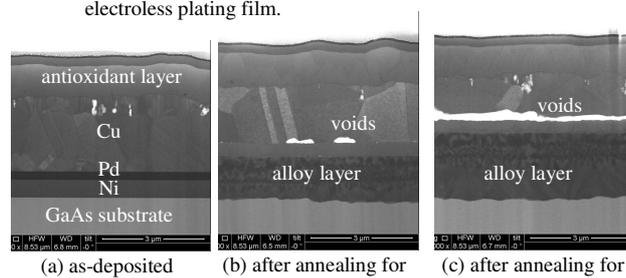
Figure 2. Cross section SEM images of the GaAs/Ni-P/Pd/Cu structure. The Pd film is the electroless plating film.
