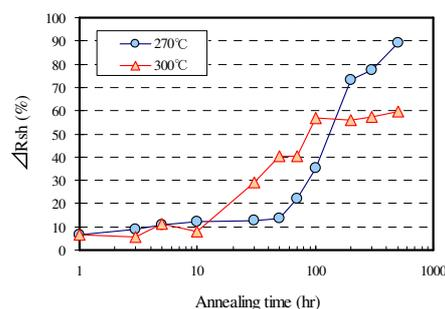
Figure 1. Sheet resistivity of the GaAs/Ni-P/Pd/Cu structure as a function of annealing time at 270°C and 300°C. The Pd film is the electroless plating film.
