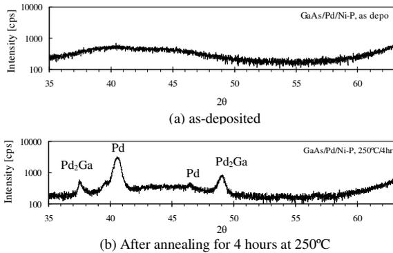
Figure 3. XRD patterns of the GaAs/Pd/Ni-P structure
