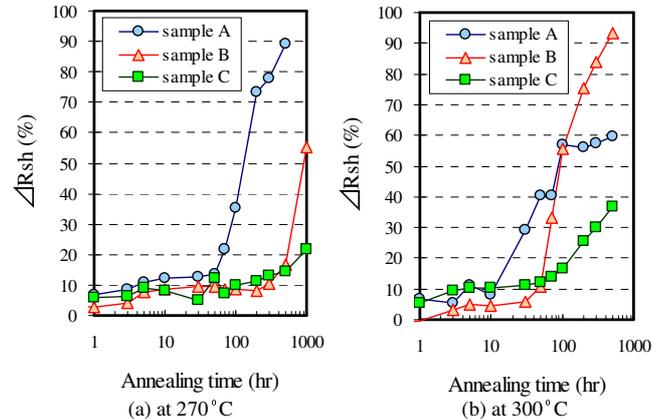
Figure 4. Sheet resistivity of samples A, B and C as a function of annealing time at 270°C and 300°C.
