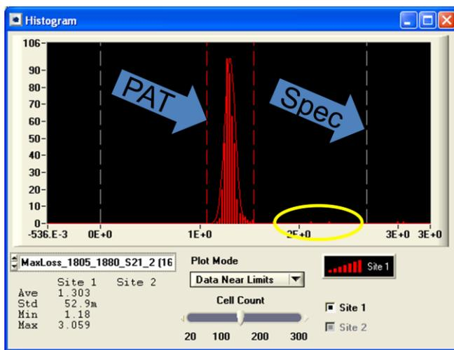
Figure 2: Devices circled passed static test limits but failed PAT limits and were effectively screen out.
