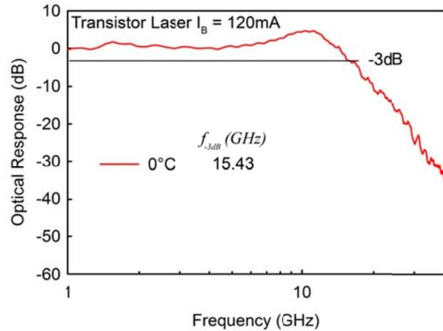
Figure 4: Frequency response of the transistor laser fabricated with the improved process showing a measured  $S_{31}$  optical response (smoothed).
