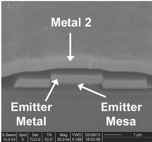
Figure 1: FIB cross-section of failed device showing discontinuity in Emitter Metal overlap due to BCB over etch.
