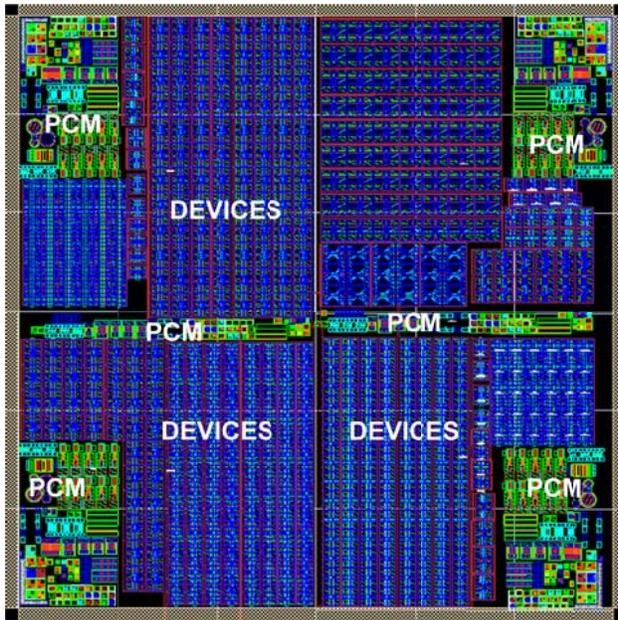
Figure 3: TL4 mask layout showing all processed layers to illustrate feature density variation across different length laser devices and PCM regions on the wafer.
