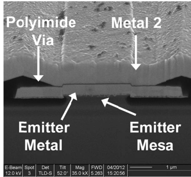
Figure 2: FIB cross-section of working device showing excellent continuity of emitter metal, sloping poly-imide vias and Metal - 2 connecting to emitter metal.
