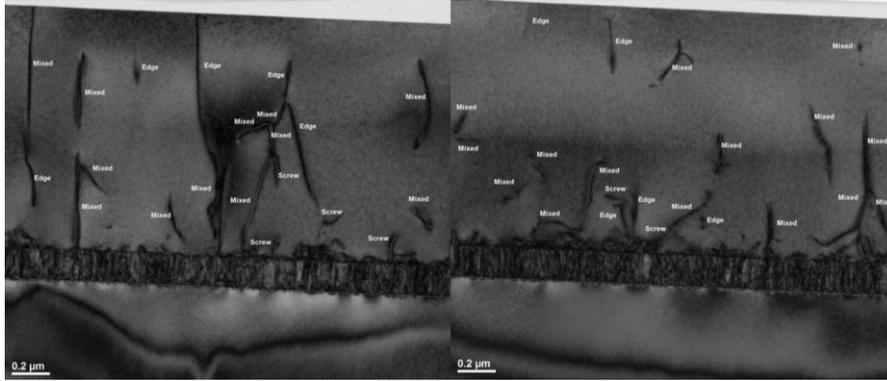
Figure 3: TEM of 1μm GaN on PVD AlN buffer. Threading defect density equals  $7 \times 10^8 / \text{cm}^2</math>$
