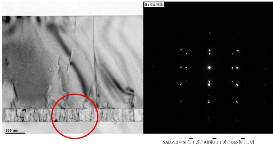
Figure 4: TEM and Diffraction Pattern of 1μm GaN on PVD AlN Buffer
