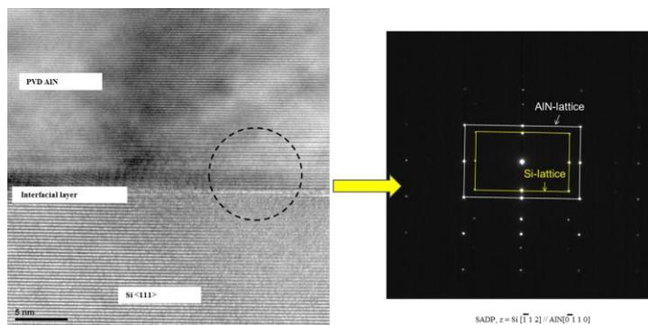
Figure 2: High Resolution, Fourier Filtered, Diffraction Micrographs by TEM
