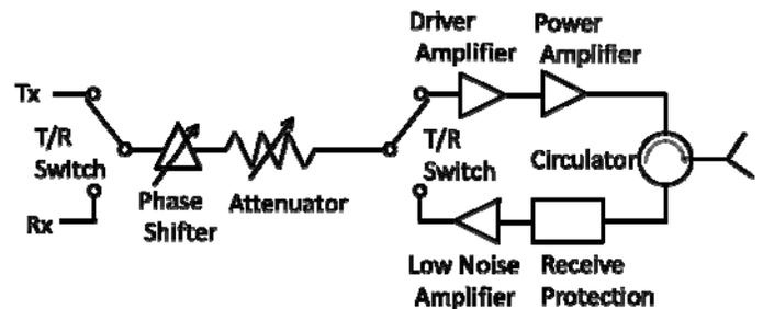
Figure 1. Block Diagram of the RF Components in a T/R Module.
