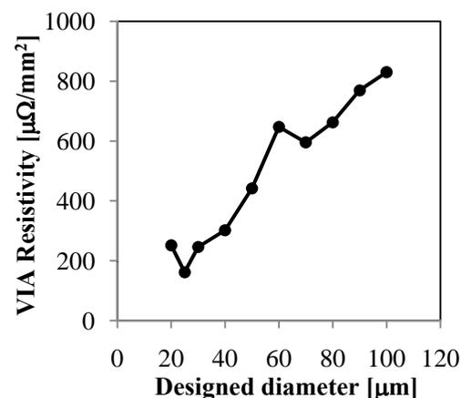
Fig. 6. Dependence of resistivity of closest formed VIAs on VIA diameter.
