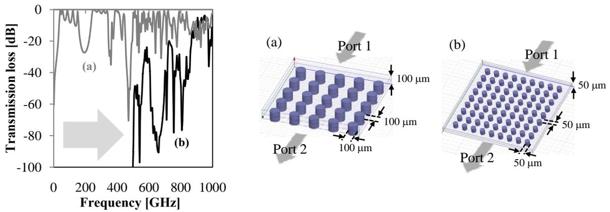
Fig. 1. Simulated fundamental mode transmission of the thinned substrate with VIAs. (a) With a 100- $\mu\text{m}$ -thick substrate and 100- $\mu\text{m}$ -gap VIAs; (b) with a 50- $\mu\text{m}$ -thick substrate and 50- $\mu\text{m}$ -gap VIAs.
