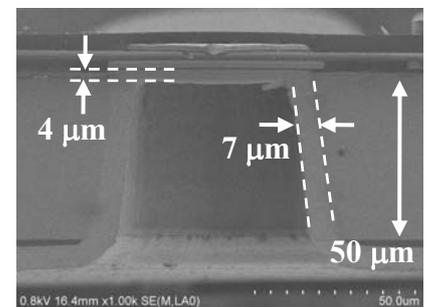
Fig. 4. Cross-sectional SEM image of Au-electroplated VIA.
