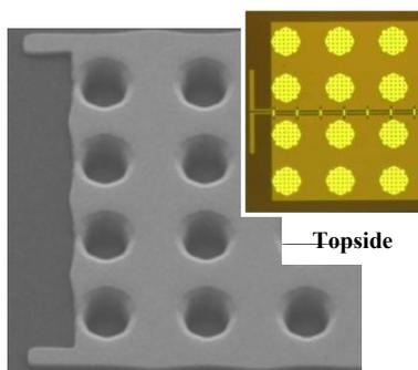
Fig. 5. Backside-patterned on-chip antenna.
