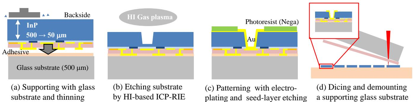
Fig. 2. Backside process flow for InP ICs.
