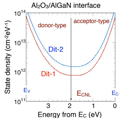
Fig. 3 Interface state density distributions used in the C–V calculation.
