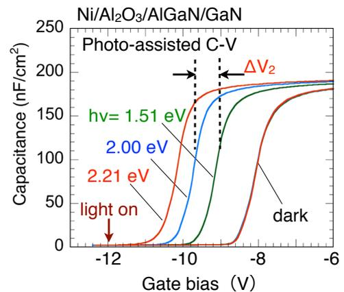
Fig. 6 Photoassisted  $C$ - $V$  characteristics of  $\text{Al}_2\text{O}_3/\text{AlGaN}/\text{GaN}$  structure.
