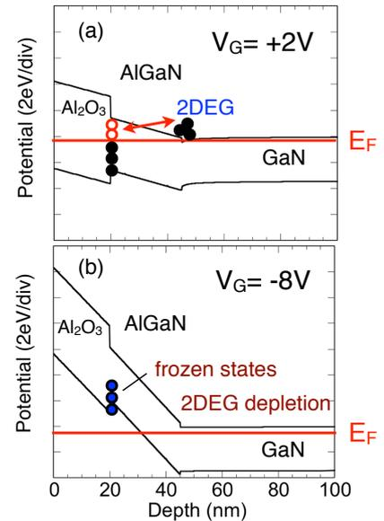
Fig. 5 Band diagram of  $\text{Al}_2\text{O}_3/\text{AlGaN}/\text{GaN}$  structure.
