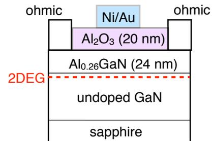
Fig. 1  $\text{Al}_2\text{O}_3/\text{AlGaN}/\text{GaN}$  structure
