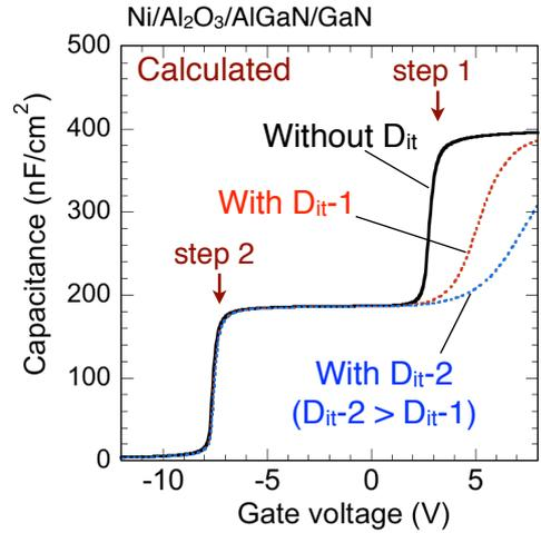
Fig. 4 Calculated  $C$ - $V$  curves of  $\text{Al}_2\text{O}_3/\text{AlGaN}/\text{GaN}$  structure.
