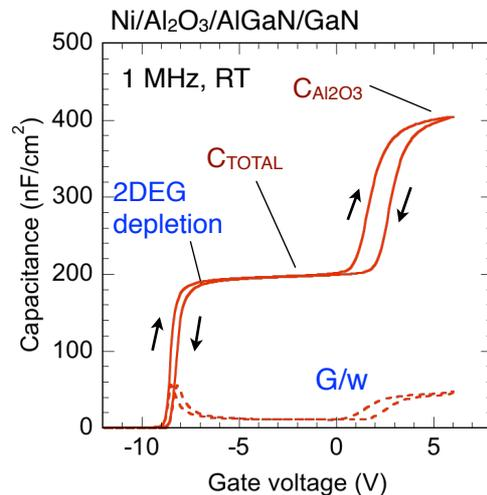
Fig. 2 Admittance characteristics of  $\text{Al}_2\text{O}_3/\text{AlGaN}/\text{GaN}$  structure.
