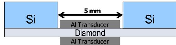
**Fig. 1. Diamond on Si wafer sample geometry used for the NCD thermal characterization measurement.**
