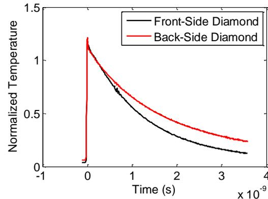
**Fig. 2. Thermal decay curve of Al on the frontside and backside the free-standing diamond window.**
