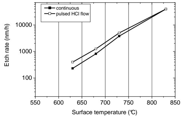
Fig. 3 Etch rates of HCl on GaN under hydrogen atmosphere (0.9 hPa). A comparison of a continuous flow of HCl and a pulsed flow is shown.
