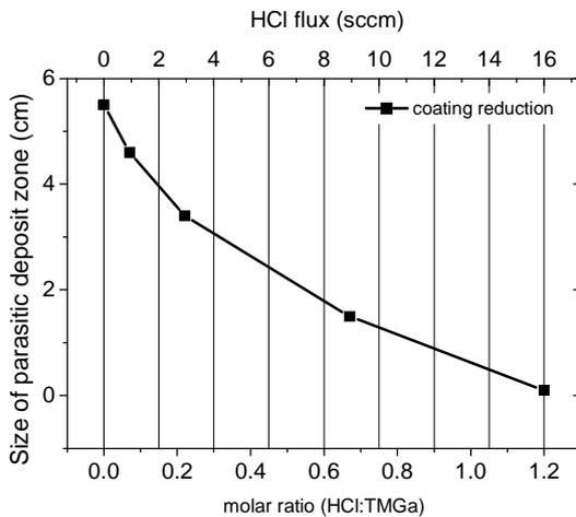
Fig 2. Reduced expansion of the parasitic deposits as a function of HCl flow. HCl is flown during growth of GaN and the distance between substrate and beginning of parasitic deposits measured.
