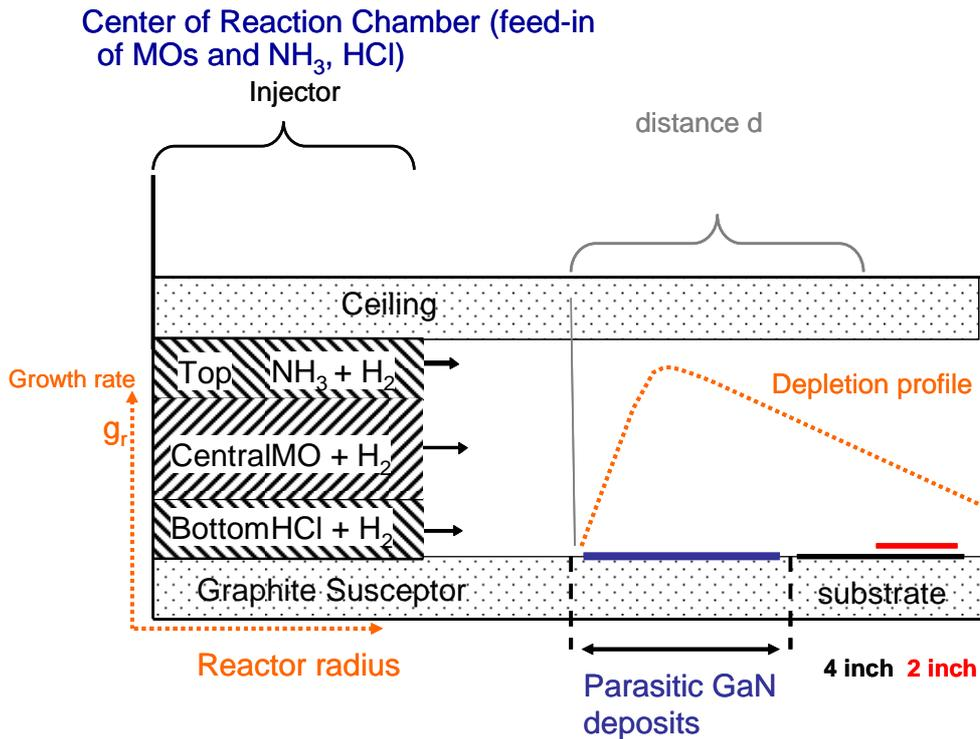
Fig 1. Experimental setup, the HCl is separated from the NH<sub>3</sub> by the central level of the injector. By introducing the HCl at the bottom level, it is introduced close to the area where the most parasitic deposits are formed. The typical depletion profile of the growth rate in a horizontal reactor is illustrated by the dotted line.
