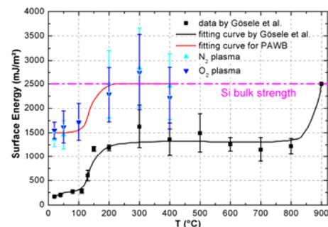
**Figure 1.** Surface energy of bonded Si/SiO<sub>2</sub> wafer pairs annealed at various temperatures for high temperature oxide bonding and plasma activated wafer bonding using N<sub>2</sub> respectively O<sub>2</sub> plasma. The maximum bond strength of 2.5J/m<sup>2</sup> is indicated by the dashed-dotted horizontal line. Data for high temperature process was taken from Ref. [1]
