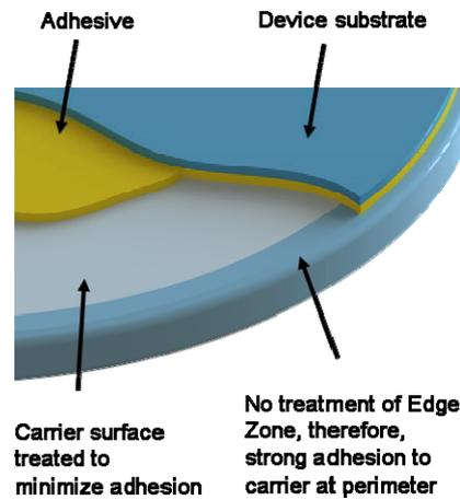
Figure 2. ZoneBOND® carrier schematic
