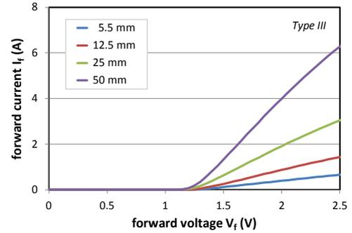
Figure 5: Forward characteristics of a Schottky barrier diode with a total device width of 5.5 to 50mm measured end-of-process on wafer C of Fig. 2.
