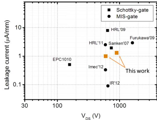
Figure 7: Benchmark on leakage current versus drain source voltage.
