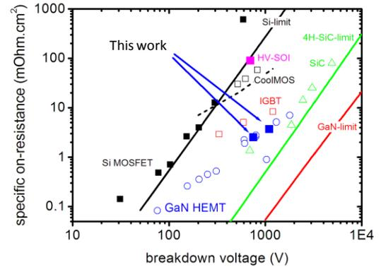
Figure 6: Benchmark on specific on-resistance versus breakdown voltage for Si, SiC and GaN devices.
