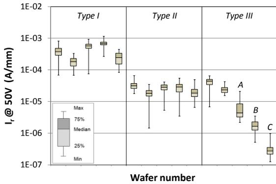
Figure 2: Evolution of Schottky reverse leakage current at  $V_{ds}=50\text{V}$  and at room temperature for 3 different process types, measured after diode formation and contact opening, showing the optimization of the Schottky module.
