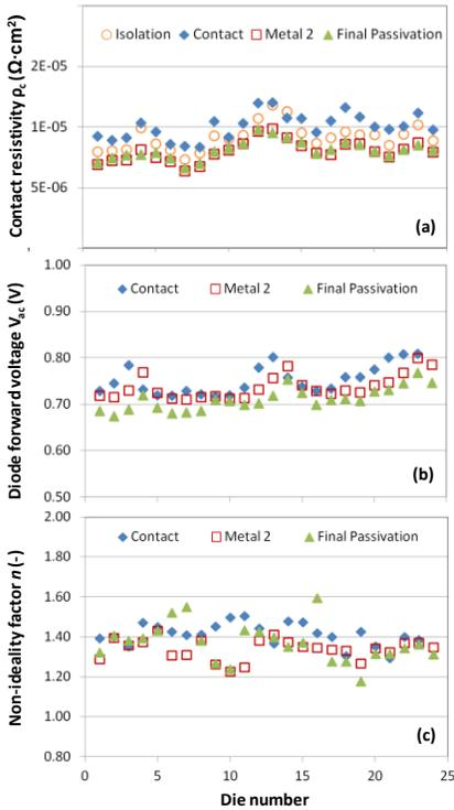
Figure 1: (a) Ohmic contact resistivity in  $\Omega\cdot\text{cm}^2$ , (b) Schottky diode forward voltage at  $0.1\text{A}/\text{cm}^2$ , (c) Schottky diode non-ideality versus die number at different stages of manufacturing.
