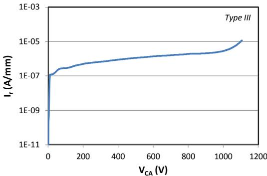
Figure 3: End-of-process Schottky reverse leakage current of a diode measured on wafer C of Fig. 2.
