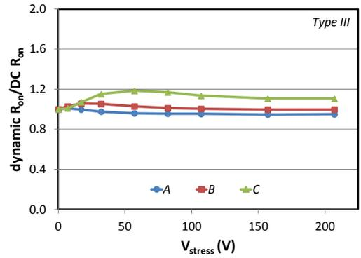
Figure 4: Ratio of dynamic  $R_{on}$  and DC  $R_{on}$ , measured end-of-process on wafers A, B and C of Fig. 2.
