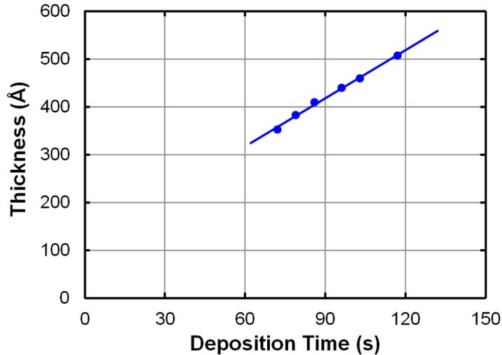
**Figure 2.** Measured PECVD  $\text{SiN}_x$  film thickness *versus* deposition time dependence derived from the location of 1<sup>st</sup> reflectance minima from the monitored multiple UV  $\text{N}_2$  plasma emission bands.
