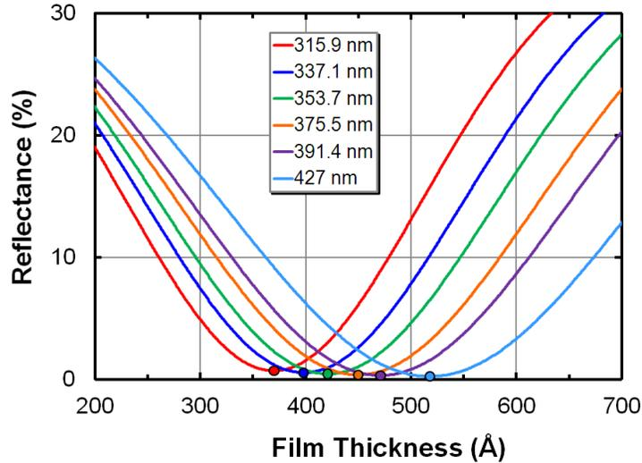
**Figure 1.** Calculated reflectance of a  $\text{SiN}_x$  film deposited on Si as function of film thickness at the indicated UV  $\text{N}_2$  plasma emission wavelengths. The symbols, (●) denote the unique film thickness at each 1<sup>st</sup> reflectance minima.
