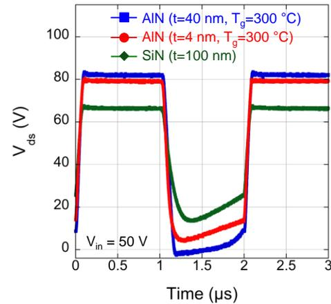
Figure 5. Drain voltage transient from boost converter test circuit on-wafer probe card for each passivation scheme. Input voltage ( $V_{in} = 50$  V), frequency = 500 kHz, duty cycle = 50%, and with a load resistor ( $R_L = 5.6$  k $\Omega$ ).
