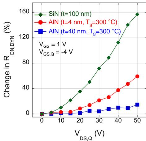
Figure 2. Increase of dynamic on-resistance of 300 °C AlN and SiN passivated AlGaIn/GaN HEMTs during pulsed measurements with increasing drain quiescent point stress ( $V_{DS,Q}$ ) in "off-state".
