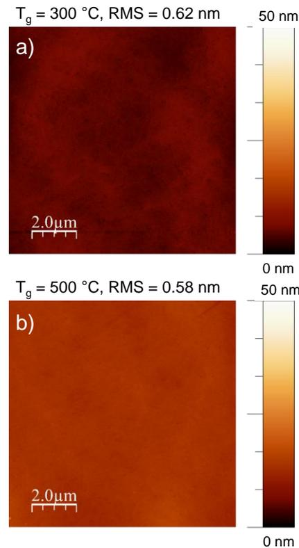
Figure 6. Surface roughness measured by AFM of ALE grown AlN films with growth temperature ( $T_g$ ) of a) 300 °C and b) 500 °C.
