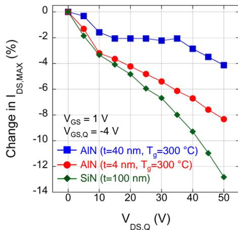
Figure 3. Reduction in  $I_{DS,MAX}$  of AlN and SiN passivated AlGaIn/GaN HEMTs during pulsed measurements with increasing "off-state" drain quiescent point stress ( $V_{DS,Q}$ ).
