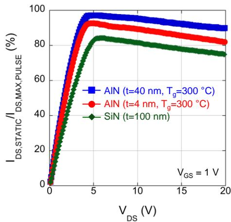
Figure 1. Current collapse for AlGaIn/GaN HEMTs passivated by AlN and SiN, shown by the ratio of collapsed DC drain current ( $I_{DS,STATIC}$ ) to the maximum drain current from pulsed I-V measurements ( $I_{DS,MAX,PULSE}$ ).
