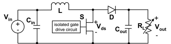
Figure 4. Block diagram of a boost converter test setup built on a probe card.
