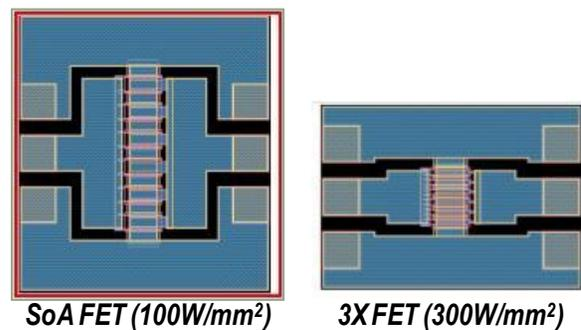
**Figure 2.** Test Vehicle Structure showing 3X Power handling improvement.
