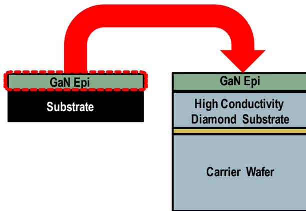
**Figure 1.** GaN epitaxial material is transferred from its growth substrate to a diamond substrate.
