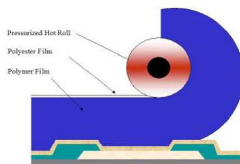
Figure 1: Dry film application using hot roll lamination
