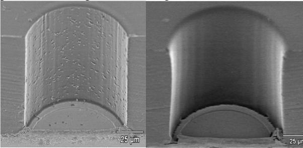
**Figure 2: Resulting photoresist via with dry film photoresist compared to spin on photoresist**
