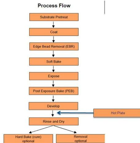
Figure 6: Process Flow
