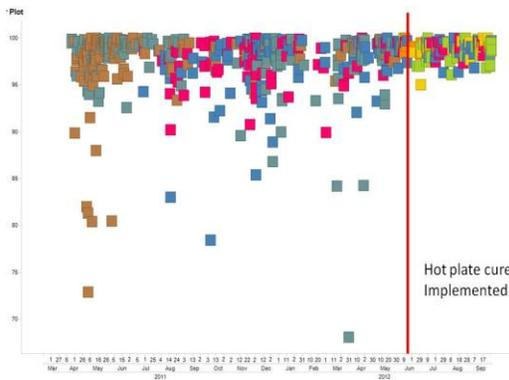
Figure 9: Final Module Yield and Hot Plate Cure
