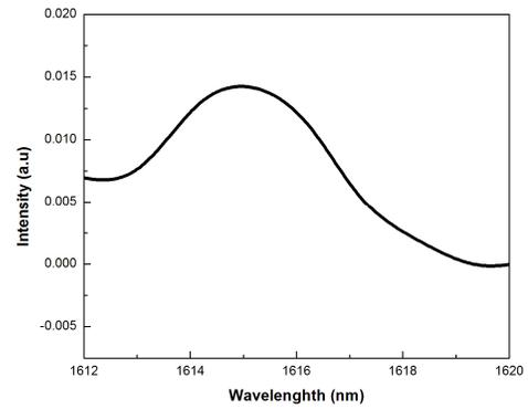
Fig 3: Photoluminescence spectra of 0.76% compressively strained 13.5 nm InGaAs QW
