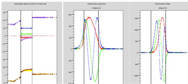
Fig.1: Self Consistent solution of schrodinger-poisson equations to determine the energy eigen values and wave functions in 13.5 nm InGaAs QW
