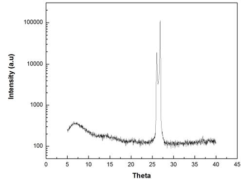
Fig 4: HRXRD to determine crystal quality
