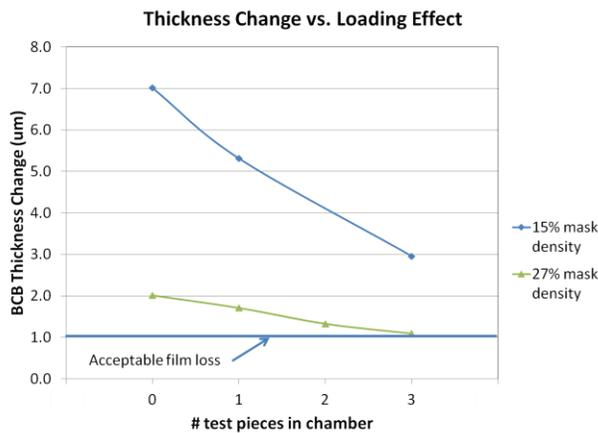
Figure 9. BCB thickness loss during plasma descum for two low density masks versus chamber loading effects.
