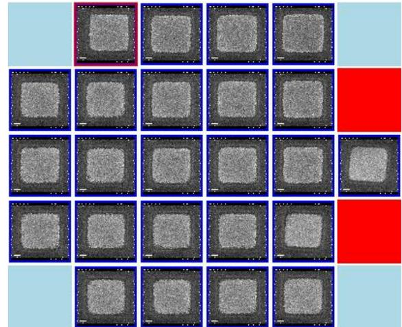
Figure 3. CDSEM wafer map of BCB openings formed using proximity exposure. This type of result was observed without exception.
