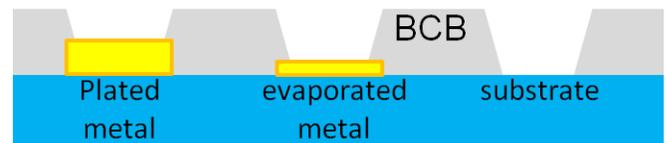
Figure 4. Due to its planarizing tendencies, the BCB thickness depends on the thickness of the local topology over which it is opened.
