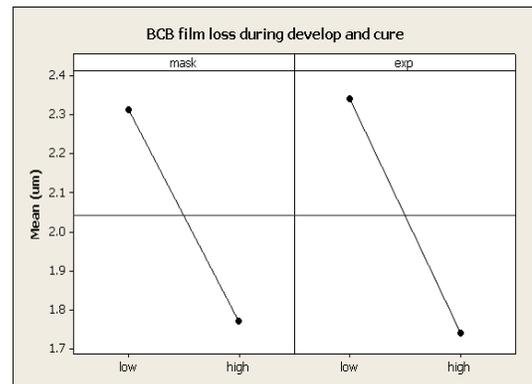
Figure 8. Average thickness loss during develop and cure as a function of mask density and exposure dose.
