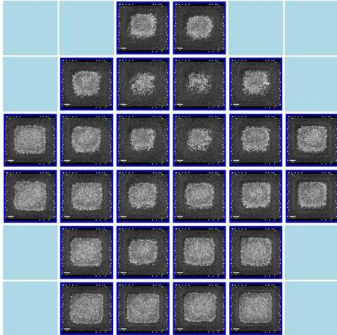
Figure 5. BCB openings to plated metal. Exposed using hard contact.
