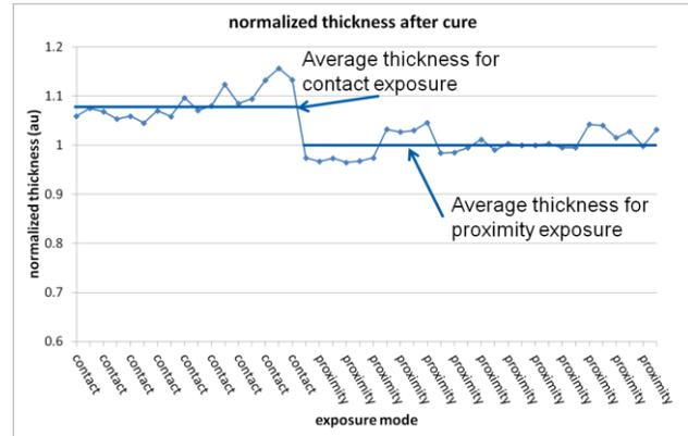
Figure 7. Because of greater film loss, BCB thickness after develop and cure is less for wafers exposed using proximity compared to those exposed using hard contact.
