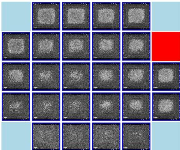
Figure 2. CDSEM wafer map of BCB openings formed using hard contact. Features were 50μm x 50μm on the mask. This result was typical although not universal.
