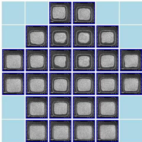
Figure 6. BCB openings to the substrate. Exposed using hard contact. Due to the thicker layer of BCB it would normally be expected that these features would be less well resolved than the openings to plated metal.
