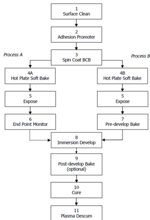
Figure 1. Photo definable BCB process flow. (From Dow Chemical product literature)
