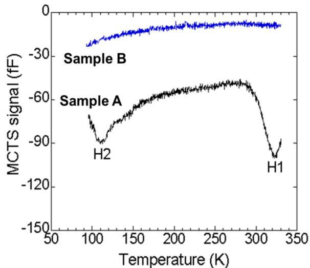
Fig.2 MCTS signals (showing hole traps) of sample A and B
