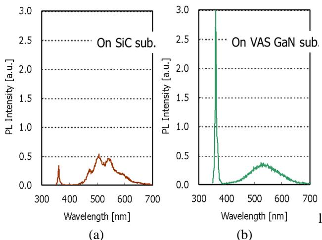
Fig.6 PL profile of GaN-HEMT-epi grown on SiC and VAS GaN substrate by same growth condition
