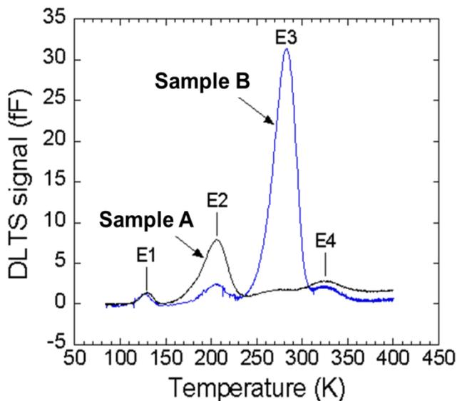
Fig.1 DLTS signals of sample A and B
