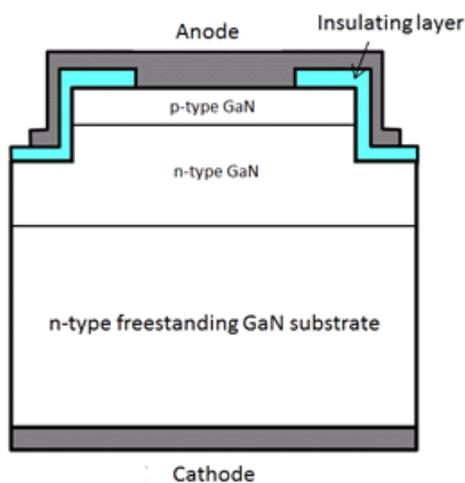
Fig.7 Cross section of P-N diode.
