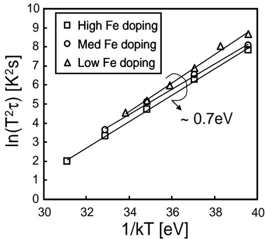
Figure 2: Activation energy extraction in the three iron-doped wafers. All the samples show consistent activation energy around 0.7 eV.
