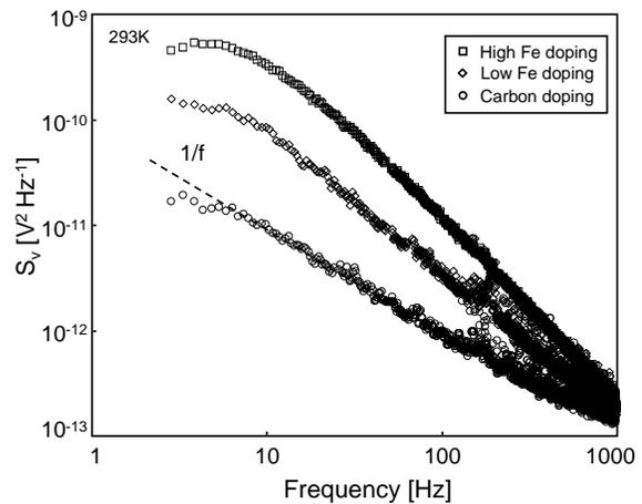
Figure 3: Low frequency noise spectra in iron- and carbon-doped AlGaIn/GaN HEMTs at room temperature. Carbon-doped devices show only 1/f behaviour while a G-R peak appears in iron-doped ones.
