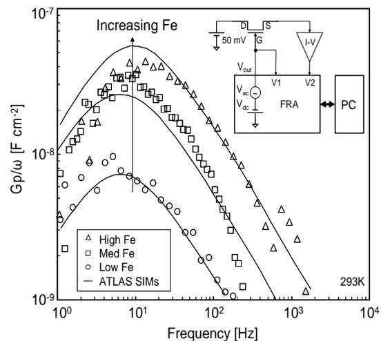
Figure 1: Measured (symbols) and simulated (solid lines) trap conductance vs. frequency at 293 K for three representative 0.25 μm AlGaIn/GaN HEMTs with different iron doping concentrations. In the inset the experimental setup is reported.
