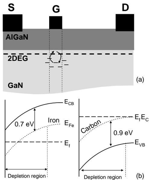
Figure 4: Schematic representation of an AlGaIn/GaN HEMT and the region probed by our measurements below the gated portion of the channel (a); Iron and Carbon trap levels: 0.7eV below the conduction band and 0.9eV above the valence band, respectively.
