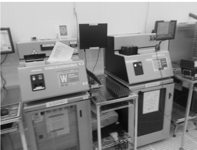
Fig. 2 Notice the differences in operating systems on these similar tools. The tool on the left still has card reader for recipe loading, while the tool on the right is updated with full automation and recipe download.
