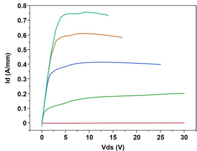
Fig. 5. Typical output characteristics of  $2 \times 50 \mu\text{m}$  devices on n-type SiC.  $V_G$  was increased in steps of 1 V from -3 V to +1V.
