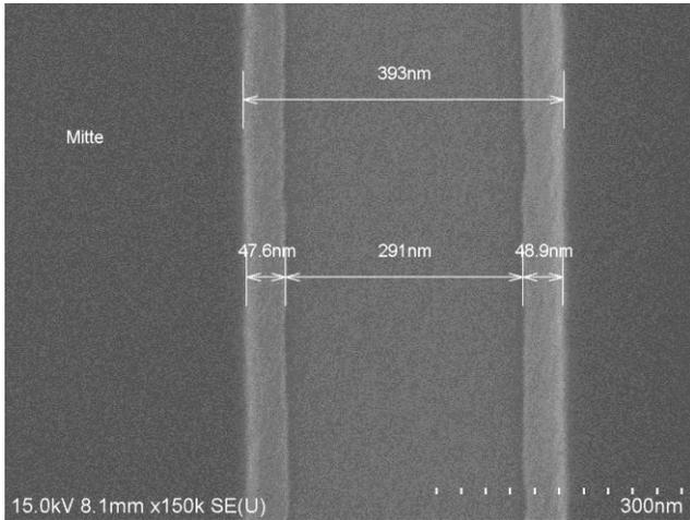
Fig. 2. Top-down SEM view of the slanted trench after combined dry and wet nitride etch
