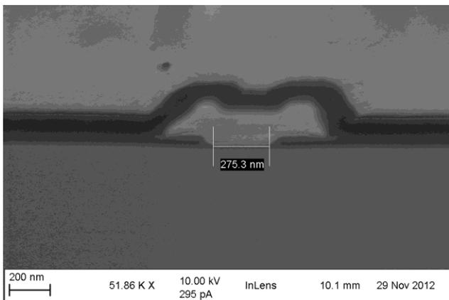
Fig. 4. FIB cross section of a metallized slanted gate on GaN wafer. The gate metal is covered by silicon nitride and a source connected field plate.
