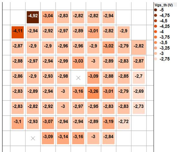
Fig. 6. Distribution of Pinch-off voltage ( $V_{gs}$  in V) across the 4<sup>x4</sup> GaN HEMT test wafer
