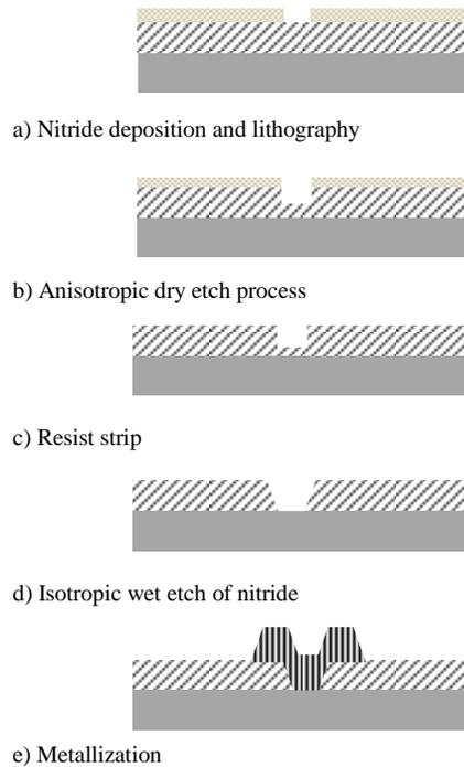
Fig. 1. Process scheme for the fabrication of slanted gates
