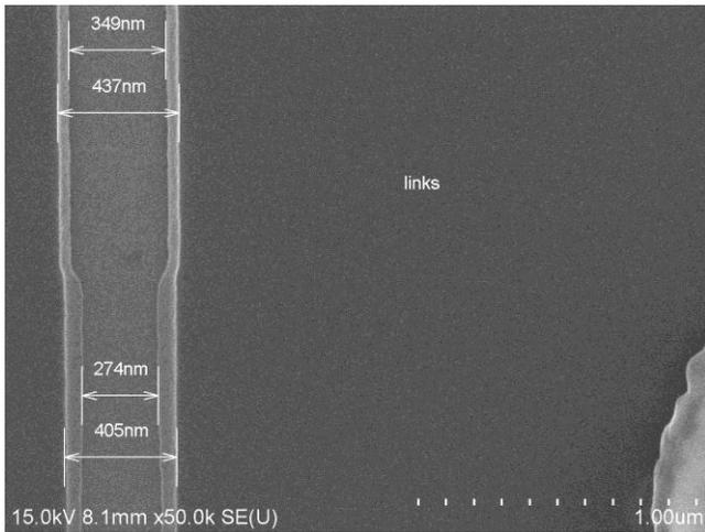
Fig. 3. Transition region implantation-no implantation after chemical etch. A widening in the implanted silicon nitride part of the trench is observed.
