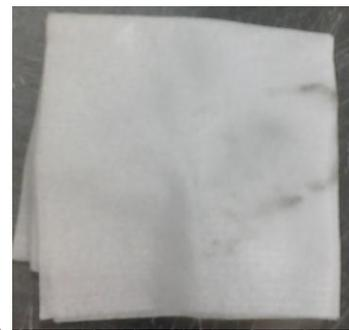
Fig. 9 Carbon residue after wiping a Au melt made from organic contaminated Au source material
