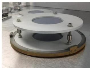
Fig. 1 Double wafer holder
