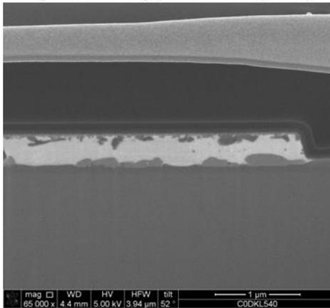
Figure 2c – SEM micrograph of 0.22 Ni fraction (290 Å Ni)
