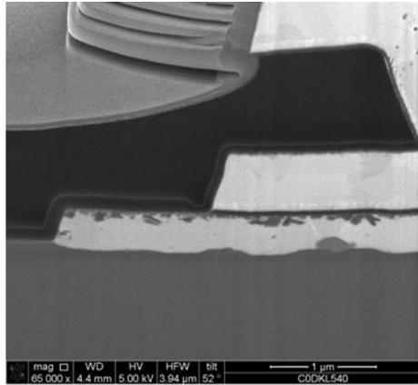
Figure 2a – SEM micrograph of 0.18 Ni fraction (230 Å Ni)
