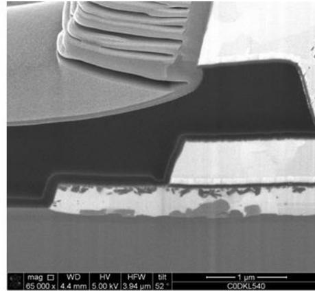
Figure 2b – SEM micrograph of 0.20 Ni fraction (260 Å Ni)
