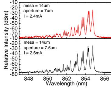
Figure 2. The emission spectra of two 7  $\mu\text{m}$  VCSEL on the same
