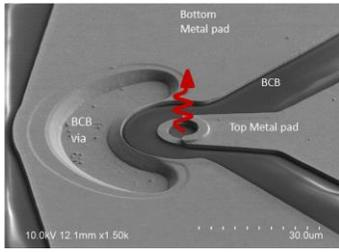
Figure 1. the SEM image of microcavity VCSEL
