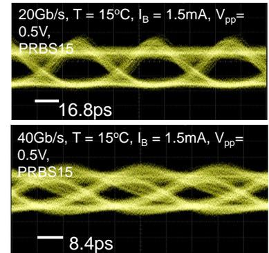
Figure 7. Eye diagrams at 20 Gb/s an 40 Gb/s data rates for 2  $\mu\text{m}$  aperture microcavity laser
