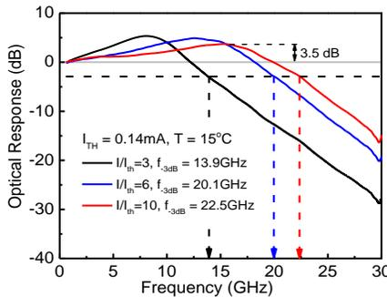
Figure 6. Frequency response of 2  $\mu\text{m}$  microcavity laser
