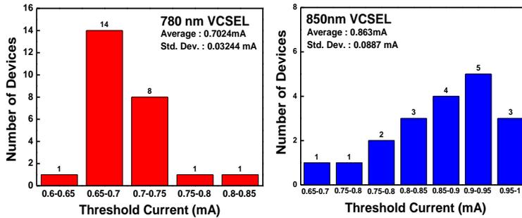
Figure 4. The threshold current distribution for 2 VCSEL
