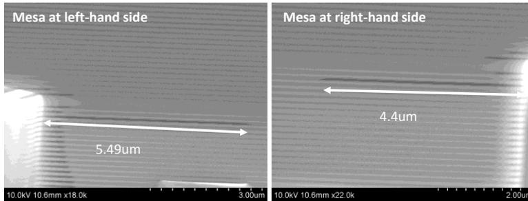
Figure 3. The cross section of a DBR mesa after oxidation in the unstable finance for 7minutes
