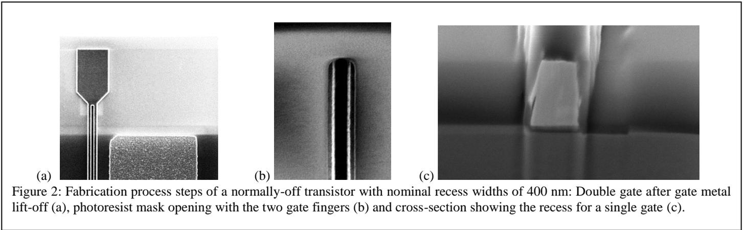
Figure 2: Fabrication process steps of a normally-off transistor with nominal recess widths of 400 nm: Double gate after gate metal lift-off (a), photoresist mask opening with the two gate fingers (b) and cross-section showing the recess for a single gate (c).
