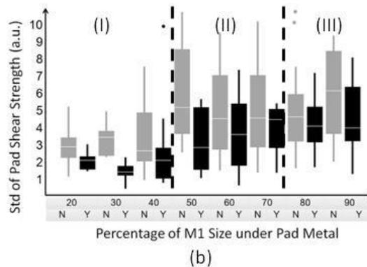
FIGURE 6 CORRELATIONS BETWEEN BUMP SHEAR STRENGTH AND NON-ANCHORED M1 UNDERNEATH PADS. (A) THE MINIMUM VALUE OF BUMP SHEAR STRENGTH AND (B) THE STANDARD VARIATION OF BUMP SHEAR STRENGTH. GRAY BOXES: PADS WITH NON-ANCHORED M1 ONLY; BLACK BOXES: PADS WITH ADDITIONAL ANCHORED M1
