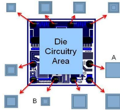
FIGURE 1 VARIATIONS OF PAD ADHESION STRENGTH WITHIN A DIE FOR DIFFERENT PADS AND ALSO WITHIN EACH PAD. THE SIZE OF THE SQUARE MARKERS OUTSIDE REPRESENTS THE ADHESION STRENGTH FOR EACH PAD
