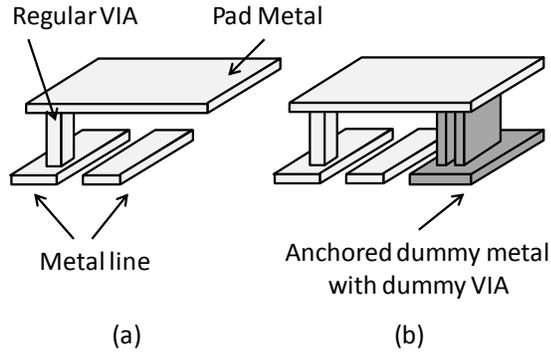
FIGURE 2 TYPICAL BOND PAD STRUCTURES CONNECTED TO A METAL LINE UNDERNEATH. (A) METAL LINES UNDER PAD METAL IN NORMAL CASES; (B) ADDITIONAL ANCHORED METAL STRUCTURE ADDED UNDER THE PAD METAL FOR MECHANICAL PAD STRENGTH IMPROVEMENT PURPOSE ONLY
