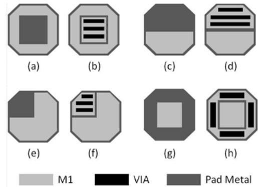
FIGURE 4 DIFFERENT LAYOUT STRUCTURES FOR PAD ADHESION STRENGTH EVALUATION WITH NON-ANCHORED M1 SIZE VARIATION AND ADDITIONAL ANCHORED M1 STRUCTURES
