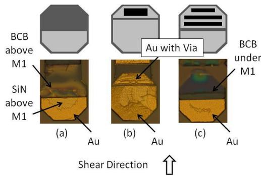
FIGURE 5 TYPICAL PAD IMAGES AFTER BUMP SHEAR. (A) A PAD WITH NON-ANCHORED M1 UNDERNEATH ONLY; (B) A PAD WITH LARGE NON-ANCHORED M1 AND ADDITIONAL SMALL ANCHORED M1; (C) A PAD WITH BOTH NON-ANCHORED M1 AND ADDITIONAL ANCHORED M1 UNDERNEATH
