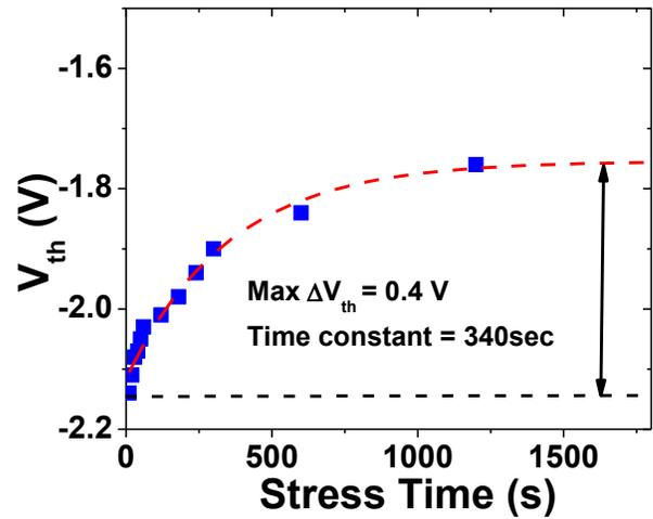
Figure 2 The relationship between the threshold voltage shift and the stress time on the AlGaIn/GaN Schottky diode.
