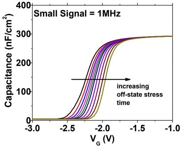
Figure 1 The measured C-V characteristics of the AlGaIn/GaN Schottky diode after different stress time.
