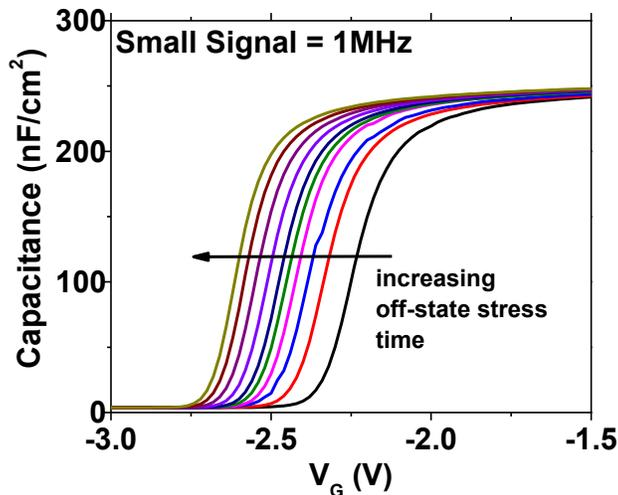
Figure 3 The measured C-V characteristics of an Al<sub>2</sub>O<sub>3</sub>/AlGaIn/GaN MIS diode after different stress time.
