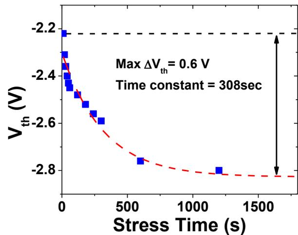
Figure 4 The relationship between the threshold voltage shift and the stress time on the Al<sub>2</sub>O<sub>3</sub>/AlGaIn/GaN MIS diode.
