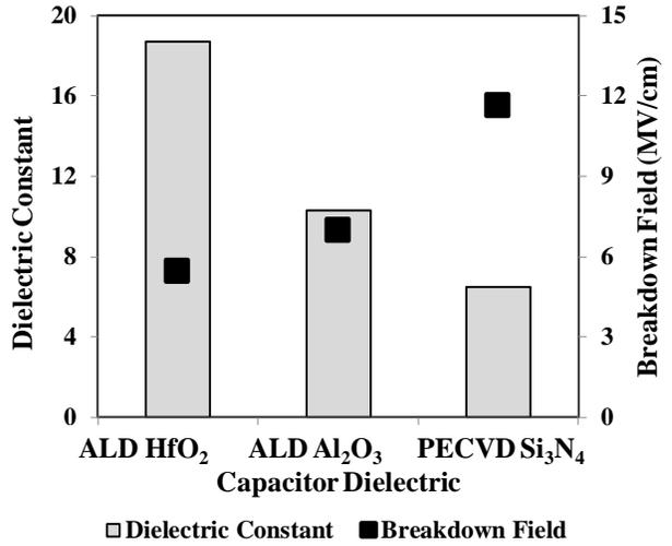
Fig 2. Dielectric constant and breakdown field of ALD HfO<sub>2</sub>, ALD Al<sub>2</sub>O<sub>3</sub>, and PECVD Si<sub>3</sub>N<sub>4</sub>.
