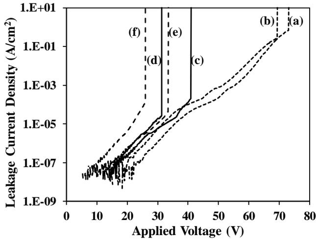
Fig 3. The I-V characteristics of GaAs MIM capacitor with capacitor dielectric 60+/-3 nm (a) PECVD Si<sub>3</sub>N<sub>4</sub> at 25°C, (b) PECVD Si<sub>3</sub>N<sub>4</sub> at 150°C, (c) ALD Al<sub>2</sub>O<sub>3</sub> at 25°C, (d) ALD Al<sub>2</sub>O<sub>3</sub> at 150°C, (e) ALD HfO<sub>2</sub> at 25°C, and (f) ALD HfO<sub>2</sub> at 150°C.
