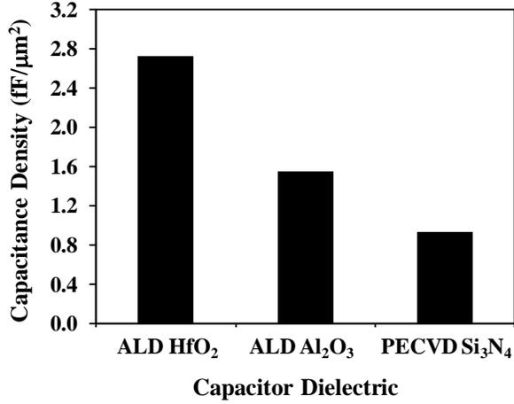
Fig 1. Capacitance density of MIM capacitor with 60+/-3 nm of ALD HfO<sub>2</sub>, ALD Al<sub>2</sub>O<sub>3</sub>, and PECVD Si<sub>3</sub>N<sub>4</sub> as capacitor dielectric on GaAs.
