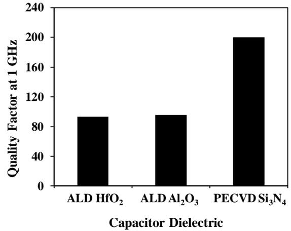
Fig 4. Quality factor of MIM capacitor with 60+/-3 nm of ALD HfO<sub>2</sub>, ALD Al<sub>2</sub>O<sub>3</sub>, and PECVD Si<sub>3</sub>N<sub>4</sub> as capacitor dielectric on GaAs.
