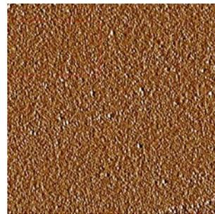
Fig. 2. AFM micrograph of NiO film (scan area 10x10  $\mu$ m) deposited in pure oxygen. Surface roughness RMS = 1.3 nm.
