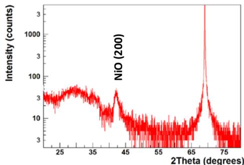
Fig. 1. X-ray diffraction patterns of 200-nm-thick NiO film deposited with RF power 2 kW in pure oxygen at pressure 3 mTorr.
