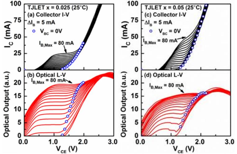
Fig. 2: (a) The collector  $I$ - $V$  characteristics and (b) Optical  $L$ - $V$  characteristics of an emitter-metal-size  $100 \times 100 \mu m^2$  TJLET (for  $In_xGa_{(1-x)}As$  tunnel junction  $x=0.025$ ). (c) The collector  $I$ - $V$  characteristics and (d) Optical  $L$ - $V$  characteristics of an emitter-metal-size  $100 \times 100 \mu m^2$  TJLET (for  $In_xGa_{(1-x)}As$  tunnel junction  $x=0.05$ ).
