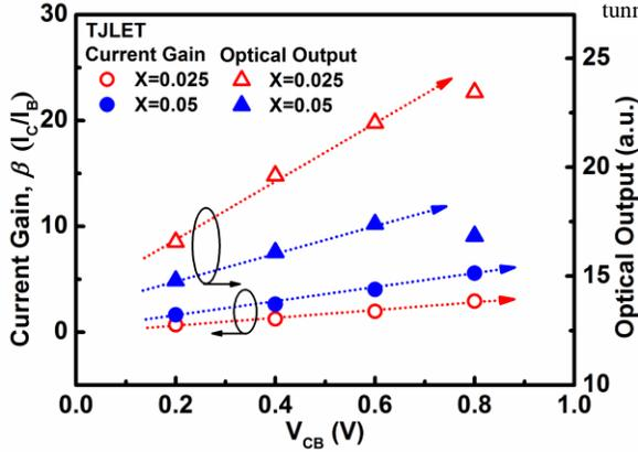
Fig. 3: The electrical current gain and optical output when BC junctions are under four different reverse-biased junction field and  $I_B=40$ mA.
