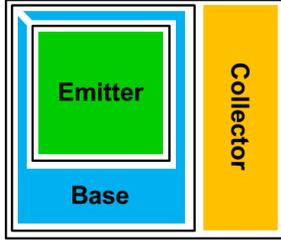
Fig. 1: Top view layout of the TJLETs.
