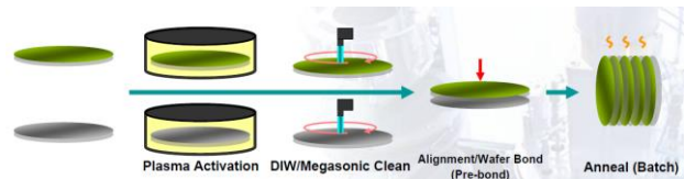
Figure 1: Fusion wafer bonding process flow
