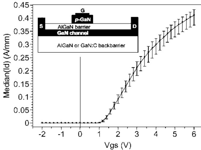
Fig.1. Transfer characteristics of p-GaN gated normally-off GaN transistors. Inset: Schematics of a normally-off transistor in p-GaN gate technology.
