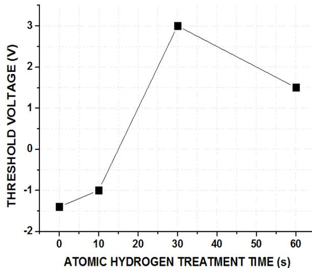
Fig. 2. Threshold voltage of p-GaN/AlGaIn/GaN transistors as a function of the treated time in the atomic hydrogen flow.
