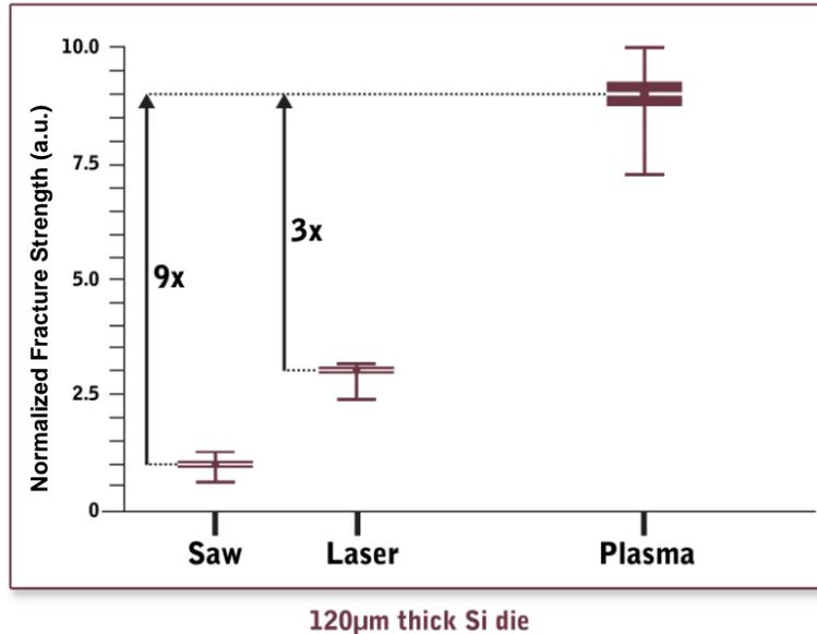
**Figure 1:** Die strength comparison between plasma, saw, and laser dicing.
