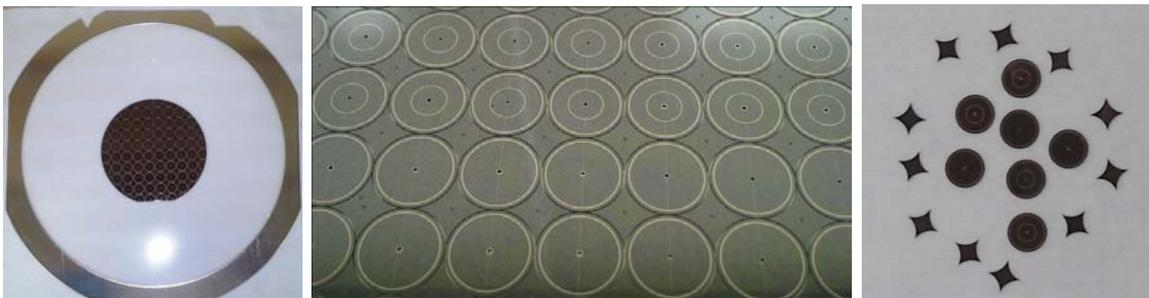
**Figure 2:** (left to right) a) 100mm wafer on dicing tape prior to etching, b) plasma dicing of circular diodes, c) fully plasma singulated devices with through wafer holes.
