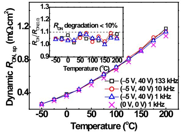
**Fig. 4:** Temperature dependence of specific dynamic  $R_{ON}$  and (inset) normalized dynamic  $R_{ON}$  at various frequencies of 1-133 kHz. Temperature of the base plate is set to be from  $-50^\circ\text{C}$  to  $200^\circ\text{C}$  in a  $25^\circ\text{C}$  step.  $R_{ON}$  extrapolated from the pulsed  $I_D$ - $V_{DS}$  curve at  $V_{GS} = 1 \text{ V}$  from  $(0 \text{ V}, 0 \text{ V})$  is used as reference.
