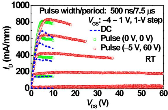
**Fig. 2:** Pulsed  $I_D$ - $V_{DS}$  characteristics (with the dc reference) from two quiescent bias points of  $(V_{GSQ}, V_{DSQ}) = (0 \text{ V}, 0 \text{ V})$  and  $(-5 \text{ V}, 60 \text{ V})$  with pulse width/period of 500 ns/7.5  $\mu\text{s}$  at RT.
