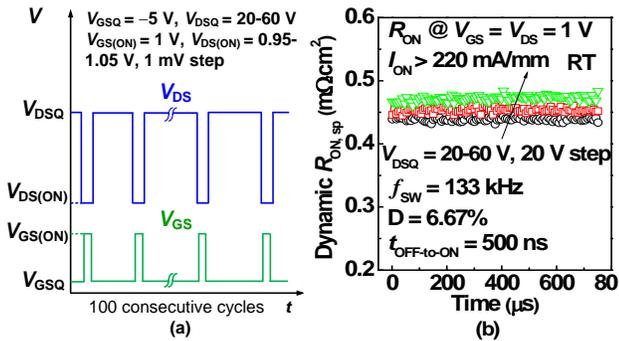
**Fig. 3:** (a) Pulsed I-V measurement setup of continuous switching test for evaluation of dynamic  $R_{ON}$  stability. (b) Time evolution of dynamic  $R_{ON}$  during 100 consecutive switching cycles at a switching frequency of 133 kHz and a duty cycle of 6.67% with an OFF-state drain bias of 20 ~ 60 V at RT.
