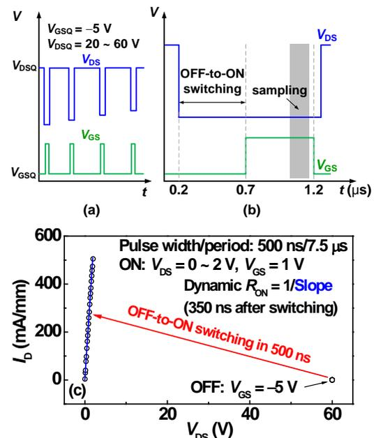
**Fig. 1:** Pulsed I-V characterizations: (a) waveforms of  $V_{GS}$  and  $V_{DS}$ ; (b) timing diagrams of  $V_{GS}$  and  $V_{DS}$  during OFF-to-ON switching (500 ns) and ON-state sampling (100 ns); and (c) dynamic  $R_{ON}$  extracted from a pulsed output curve in the linear regime. The pulse width and period are 500 ns and 7.5 μs, respectively. The data were recorded 350 ns after switching.
