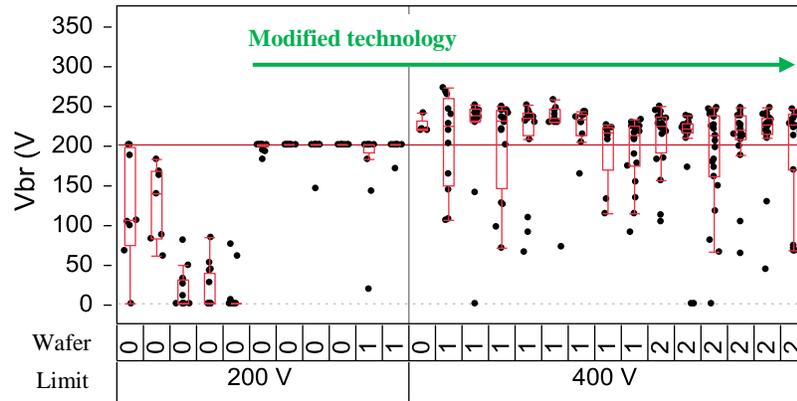
Figure 3. Box-and-whisker plots of MIM capacitor breakdown measurements performed on wafers 01-05 processed before modification and 20 wafers (06-25) processed in 5 consecutive process runs after modification of technology. The measurements were limited by 200 V and 400 V as represented by two groups of plots. The current limit is 10  $\mu$ A.
