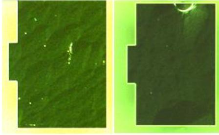
Figure 2. Dark field light microscopy images of the MIM bottom plates showing particles, scratches and epitaxial defects as spots with increased intensity.
