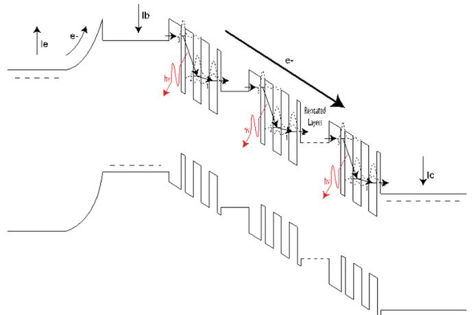
Figure 1. Band diagram illustration in a TI-QCL.
