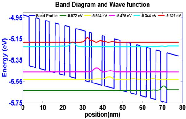
Figure 2. Active region and injector design in the quantum cascade region in TI-QCL. The lasing wavelength shown in the figure is  $8.05\mu\text{m}$ .
