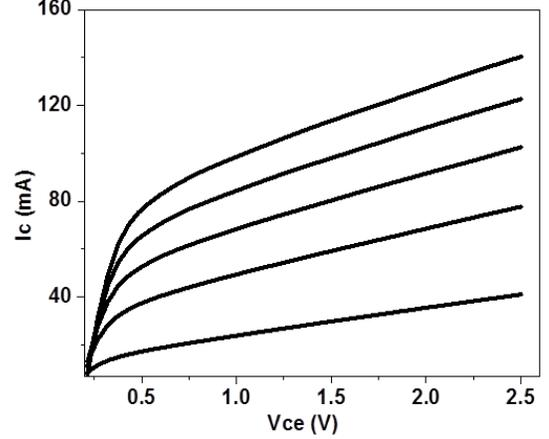
Figure 4. The transistor family of curves of the TI-QCL. The collector currents vs. the collector-emitter voltage are plotted.
