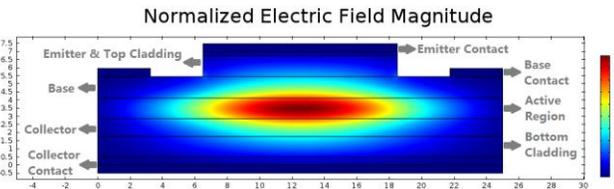
Figure 3. Normalized electric field magnitude in a cross section of TI-QCL. From the top: contact, top cladding layer, emitter, base, active region, collector, subcollector, bottom cladding layer, bottom contact.
